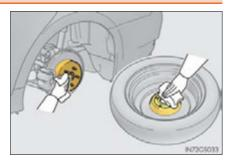
**2** Install the spare tire and loosely tighten each wheel nut by hand by approximately the same amount.
