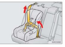
**6** If the child restraint has a top tether strap, the top tether strap should be latched onto the top tether strap anchor. ( $\rightarrow$ P. 66)
