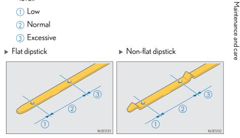
The shape of the dipstick may differ depending on the type of vehicle or engine.
