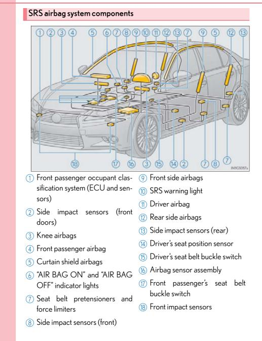
Your vehicle is equipped with ADVANCED AIRBAGS designed based on the US motor vehicle safety standards (FMVSS208). The airbag sensor assembly (ECU) controls airbag deployment based on information obtained from the sensors etc. shown in the system components diagram above. This information includes crash severity and occupant information. As the airbags deploy, a chemical reaction in the inflators quickly fills the airbags with non-toxic gas to help restrain the motion of the occupants.
