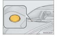
When the light switch is in AUTO or ED: The headlights and tail lights turn off 30 seconds after the engine switch is turned to ACCESSORY mode or turned off and a door is opened and all of the doors and trunk are closed. (The lights turn off immediately if **a** on the key is pressed twice after all the doors are closed.)
