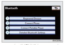
To display the screen shown above, press the "MENU" button on the Remote Touch, then select "Setup", select "Bluetooth\*" on the "Setup" screen.
