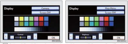
Select "<" or ">" to select the desired function ("Contrast" or "Brightness") and then select the desired screen button to adjust contrast and brightness.
