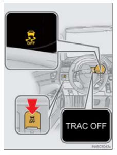
When the message is displayed on the multi-information display showing that TRAC has been disabled even if the VSC OFF switch has not been pressed
