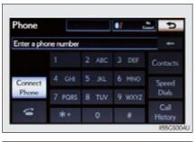
3 Select the screen button corresponding to the desired phone connection.
