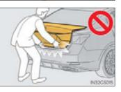
• Do not attach any accessories other than genuine Lexus parts to the trunk lid. Such additional weight on the trunk lid may cause the lid to suddenly shut again after it is opened.
