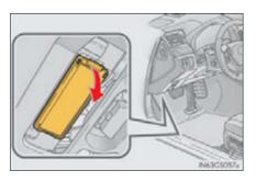
Passenger's side instrument panel Remove the lid.
