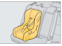
3 Open the anchor bracket cover, latch the hook onto the anchor bracket and tighten the top tether strap.
