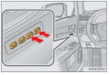
Vehicles with the driving position memory for the front passenger's seat: To record the position of the front passenger's seat, adjust the front passenger's seat to the desired position and perform step 4 using the buttons on the front passenger's side.
