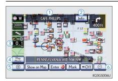
To scroll over the map, place the pointer in a position near the desired destination and then press and hold Remote Touch knob.
