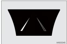
The inside of the recognized lane line turns white when the right or left lane marker is recognized.
