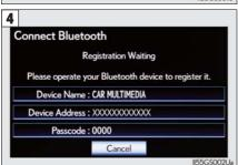
To use a Bluetooth<sup>®</sup> phone, it is necessary to first register it in the system.
