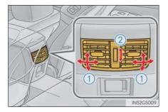
Fan speed is adjusted automatically according to the temperature setting and the ambient conditions.
