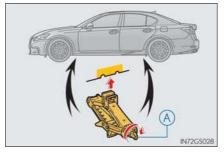
A Raise the vehicle until the tire is slightly raised off the ground.
