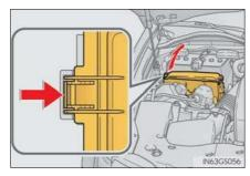
► Engine compartment (type B fuse box)
