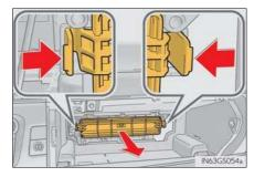
The "↑UP" marks shown on the filter and the filter case should be pointing up.
