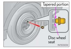
When replacing an aluminum wheel with an aluminum wheel, turn the wheel nuts until the washers come into contact with the disc wheel.
