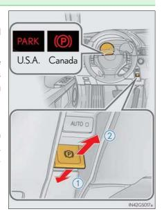
The parking brake is set or released automatically according to shift lever operation.
