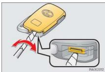
Remove the depleted battery.
