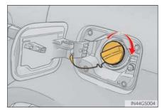
2 Close the fuel filler door, and press the center of the rear edge of the fuel filler door until you hear a click.
