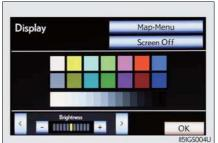
3 Select "<" or ">" to select the desired function ("Contrast" or "Brightness") and then select the desired screen button to adjust contrast and brightness.
