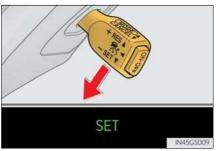
To change the set speed, operate the lever until the desired set speed is displayed.
