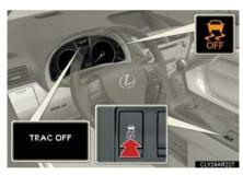
To turn the TRAC and VSC systems off, press and hold the switch for more than 3 seconds while the vehicle is stopped.
