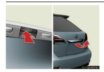
To open the back door, push up the opener button and raise the door.
