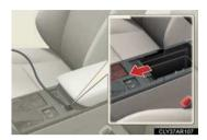
When the cover is slide open, accessory device cables can be pulled through the opening.
