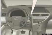
Press the "ENGINE START STOP" switch.
