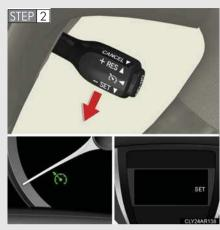
Accelerate or decelerate to the desired speed, and push the lever down to set the speed.
