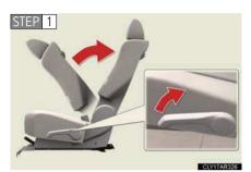
Fold the seatback while pulling the seatback angle adjustment lever. Return the seatback and secure it at the first lock position. (→P. 66)
