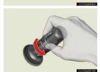
Intermittent operation: Wiper interval can be adjusted by turning the band.
