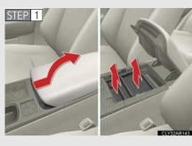
Slide the armrest while pulling up the lever, and lift the armrest. Remove the upper trays (if equipped).
