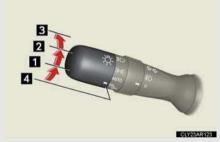
The headlights and side marker, parking, tail, license plate, daytime running lights and instrument panel lights turn on and off automatically (when the "ENGINE START STOP" switch is in IGNITION ON mode).
