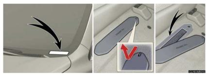
This number is stamped on the top left of the instrument. On some models, this number is also stamped under the front passenger seat.
