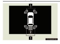
Sensors are used to detect obstacles near the vehicle. The distance to a detected obstacle is shown by the number of indicator bars.
