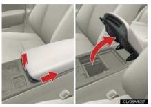
Slide the armrest while pulling up the lever, and lift the armrest.
