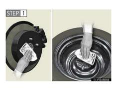
Remove any dirt or foreign matter from the wheel contact surface.
