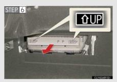
To remove the filter case, lift it up and pull it out. Replace the filter with a new one.
