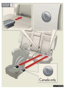
Latch the buckles onto the LATCH anchors. If the child restraint has a top tether strap, the top tether strap should be latched onto the top tether strap anchor bracket.
