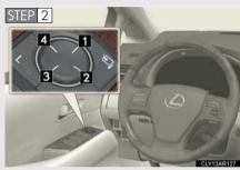
To adjust the mirror, press the switch.
