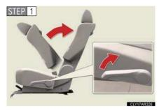
Fold the seatback while pulling the seatback angle adjustment lever. Return the seatback and secure it at the first lock position.  $(\rightarrow P. 66)$
