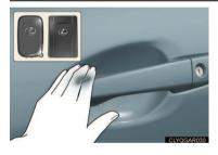
To lock the vehicle, touch the lock sensor on either of the front door handles.
