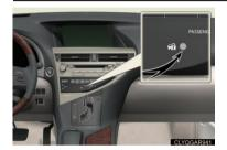
The engine immobilizer system prevents the engine from being started in the event that an attempt is made to start the vehicle using an unregistered key.
