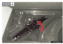
Remove the jack after removing the hook.
