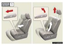
Move the front seat forward, raise the seat, and remove the head restraint ( $\rightarrow$ P. 73).
