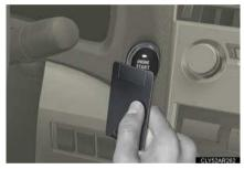
STEP 3 To change "ENGINE START STOP" switch modes: Within 10 seconds of the buzzer sounding, release the brake pedal and press the "ENGINE START STOP" switch. Modes can be changed each time the switch is pressed. (→P. 154)
