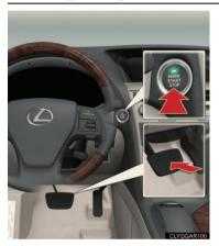
Make sure the parking brake is set and the shift lever is in P.
