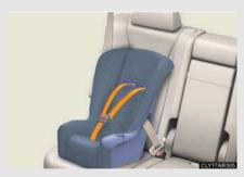
Seat belts equipped with a child restraint locking mechanism (ALR/ELR belts except driver's seat belt) (→P.75)
