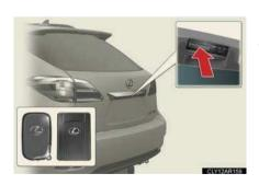
Press the button to unlock the door.
