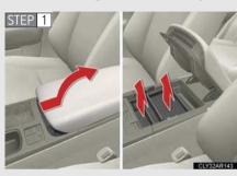
Slide the armrest while pulling up the lever, and lift the armrest. Remove the upper trays (if equipped).
