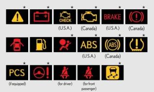
\*: These lights turn on when the "ENGINE START STOP" switch is turned to IGNITION ON mode to indicate that a system check is being performed. They will turn off after the engine is started, or after a few seconds. There may be a malfunction in a system if a light does not come on, or if the lights do not turn off. Have the vehicle inspected by your Lexus dealer, for details.
