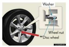
Turn the nuts until the washers come into contact with the wheel.
