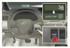
Pressing and holding the head-up display main switch for more than 2 seconds changes the display to audio display on/off mode. Press the head-up display main switch to turn the audio display on/off.
