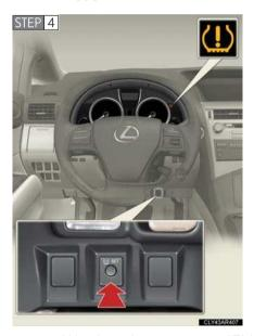
Press and hold the tire pressure warning reset switch until the tire pressure warning light flashes slowly 3 times.
