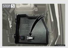
Remove the fuse with the pullout tool.
