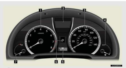
■ Tachometer Displays the engine speed in revolutions per minute
