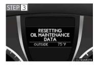
Keep the "ODO/TRIP" button pressed for about 5 seconds. The resetting procedure is complete when "OOOOO" in the trip meter flashes once and the message in the multi-information display disappears.
