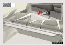
Attach the hooks to the hook brackets on the rear seat seat-back.
