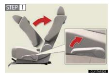
Fold the seatback while pulling the seatback angle adjustment lever. Return the seatback and secure it at the first lock position.  $(\rightarrow P. 66)$
