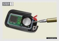
Remove the depleted battery.
