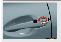
To unlock or lock the vehicle, use the mechanical key. (driver's door only) The mechanical key is stored inside the electronic key.
