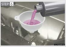
Add engine coolant if necessary.
