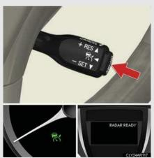
Selecting vehicle-to-vehicle distance control mode:
