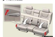
Pull the seatback angle adjustment lever.
