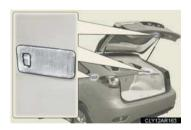
The luggage compartment lights turn on when the back door is opened with the luggage compartment light switch on.
