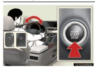
The steering wheel locks when the "ENGINE START STOP" switch is turned off and the driver's door is opened.
