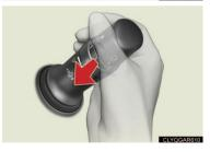
To spray washer fluid, pull the lever. The wipers will operate automatically.
