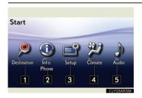
Press the "MENU" button on the Remote Touch to display the "Start" screen.
