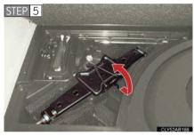
Remove the jack after removing the hook.
