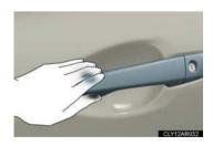
Touch both lock sensors on the upper and lower part of the door handle simultaneously.
