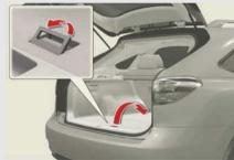
Pull the lever upwards when lifting the deck board up.
