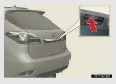
When the back door is unlocked: Press the back door opener button.
