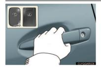
To unlock the vehicle, simply grasp either of the front door handles.
