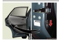
Pushing down the switch prevents the rear doors from being opened from the inside.
