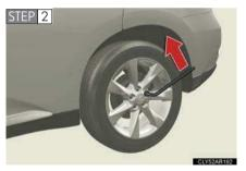
Slightly loosen the wheel nuts (one turn).
