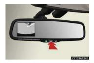
When the screen is displayed, press the "AUTO" button on the inside rear view mirror to switch the screen on/off
