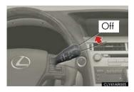
Set the wiper switch to the off position. If the wiper switch is in "AUTO", the wipers may operate and the wiper blades may be damaged.
