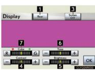
Press the "DISP" button on the Remote Touch to show the "Display" screen.
