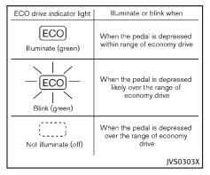
When the ECO drive indicator illuminates in green, the accelerator reaction force is normal. When the ECO drive indicator light is blinking or remains off, the ECO pedal system increases the reaction force of the accelerator pedal.
