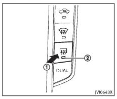
To defog/defrost the rear window glass and outside mirrors, start the INFINITI Direct Response Hybrid<sup>®</sup> System and push the switch ① on. The indicator light ② will come on. Push the switch again to turn the defroster off.
