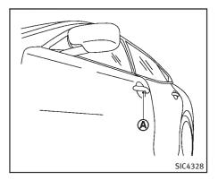
When the doors are unlocked by pushing the UNLOCK button on the Intelligent Key or touching the one touch unlock sensor with the ignition switch in the LOCK position, the courtesy light (A) will illuminate.
