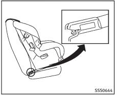
LATCH rigid-mounted attachment The child restraint top tether strap must be used when installing child restraints with the LATCH lower anchor attachments or seat belts. (See "Installing top tether strap" (P.1-33).)
