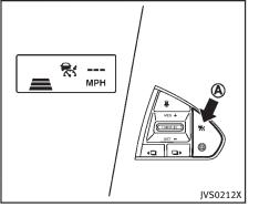
Operating vehicle-to-vehicle distance control mode
