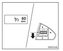
**To set cruising speed,** accelerate your vehicle to the desired speed, push the SET/COAST (-) switch and release it. (The color of the cruise indicator changes to green and set vehicle speed indicator comes on.) Take your foot off the accelerator pedal. Your vehicle will maintain the set speed.
