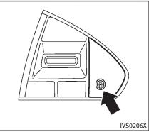
**Dynamic driver assistance switch** Active Lane Control turns on when the dynamic driver assistance switch on the steering wheel is pushed and [Active lane control] and [Lane Departure Prevention] are enabled in the settings menu on the lower display. See "How to enable/disable the LDP system" (P.5-35).
