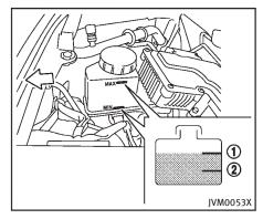
Check the fluid level in the reservoir. If the fluid is below the MIN line ② or the brake warning light comes on, add Genuine NISSAN Super Heavy Duty Brake Fluid or equivalent **DOT 3** fluid up to the MAX line ①. If fluid must be added frequently, the system should be checked by an INFINITI retailer.
