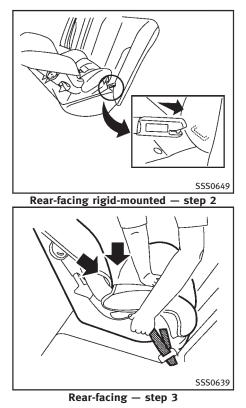
3. For child restraints that are equipped with webbing-mounted attachments, remove any additional slack from the anchor attachments. Press downward and rearward firmly in the center of the child restraint with your hand to compress the vehicle seat cushion and seatback while tightening the webbing of the anchor attachments.
