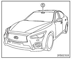
Active Lane Control slightly corrects front tire angles and steering wheel torque to help reduce the difference between the vehicle's direction and the lane direction (2) which is detected by using the camera unit (1) located above the inside mirror.
