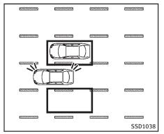
If the driver activates the turn signal, then the side indicator light flashes and a chime will sound twice.
