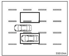
If the BSI system is on and your vehicle is approaching a lane marker, the side indicator light flashes and a chime will sound three times. Then the BSI system slightly applies the steering to help return the vehicle back to the center of the driving lane.
