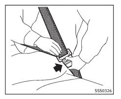
• Grasp the shoulder belt and pull forward quickly. The retractor should lock and restrict further belt movement. If the retractor does not lock during this check or if you have any question about seat belt operation, see an INFINITI retailer.
