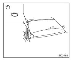
Be sure not to put anything on top of the photo sensor ① located on the top of the instrument panel. The photo sensor controls the autolight; if it is covered, the photo sensor reacts as if it is dark and the headlights will illuminate.
