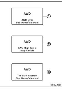
If the "AWD Error" warning ① appears, there may be a malfunction in the Intelligent AWD system. Reduce vehicle speed and have your vehicle checked by an INFINITI retailer as soon as possible.
