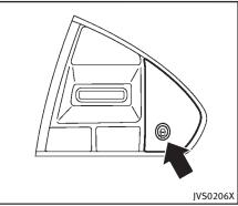
**Dynamic driver assistance switch** The LDP system turns on when the dynamic driver assistance switch on the steering wheel is pushed when the [Lane Departure Prevention] is enabled in the settings menu on the lower display. The driver assist system lane indicator (green) illuminates in the vehicle information display when the LDP system is turned on.
