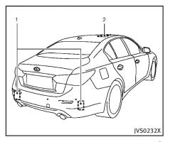
The BSW system uses radar sensors ① installed near the rear bumper to detect other vehicles in an adjacent lane. In addition to the radar sensors, the BSI system uses a camera ② installed behind the windshield to monitor the lane markers of your traveling lane.
