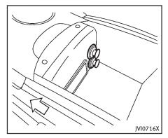
The power outlets are located in the center console.
