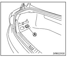
The 12-volt battery (A) is located on the left hand side of the trunk behind an access panel.
