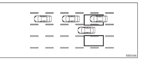
If the BSI system is on and your vehicle approaches a lane marker while another vehicle is in the detection zone, the side indicator light flashes and a chime will sound three times. Then, the BSI system slightly applies the steering to help return the vehicle back to the center of the driving lane.
