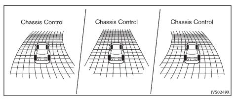
When the active trace control is operated and the "Chassis Control" mode is selected in the trip computer, the active trace control graphics are shown in the vehicle information display. (See "Trip computer" (P.2-31).)
