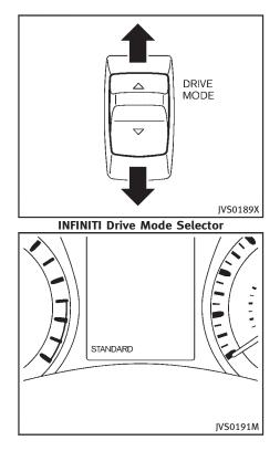
Five driving modes can be selected by using the INFINITI Drive Mode Selector (PERSONAL, SPORT, STANDARD, ECO and SNOW).
