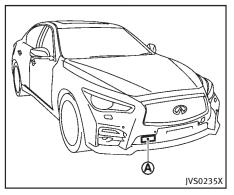
The forward emergency braking system uses a radar sensor (A) located behind the lower grille of the front bumper to measure the distance to the vehicle ahead in the traveling lane.
