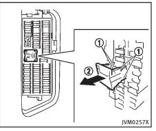
Extended storage fuse switch (if so equipped)
