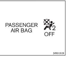
7. If the booster seat is installed in the front passenger seat, push the ignition switch to the ON position. The front passenger air bag status light shared may or may not illuminate depending on the size of the child and the type of booster seat used. See "Front passenger air bag and status light" (P.1-44).
