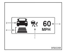
ICC system display and indicators The display is located between the speedometer and tachometer.
