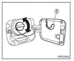
To remove the fuel-filler cap:
