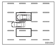
If the BSI system is on and your vehicle approaches the lane marker while another vehicle is in the detection zone, the side indicator light flashes and a chime will sound three times. Then, the BSI system slightly applies the steering to help return the vehicle back to the center of the driving lane.
