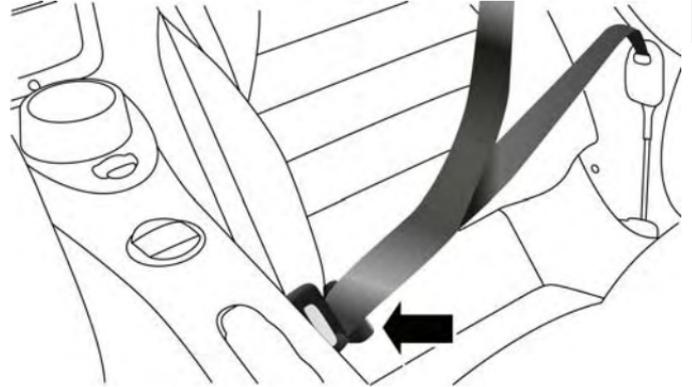
**Inserting Latch Plate Into Buckle**
