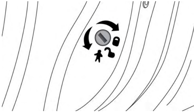
Child-Protection Door Lock Location
