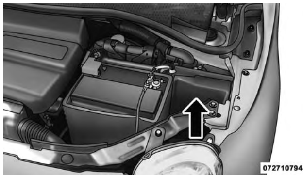
Front Distribution Unit
