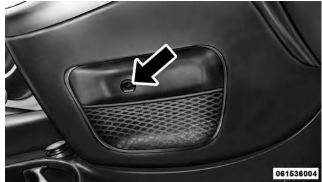
Shift Lever Override Access Hole
