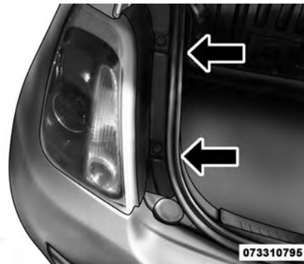
Tail Lamp Assembly Screws
