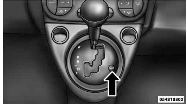
ESC Off Switch (Automatic Transmission)
