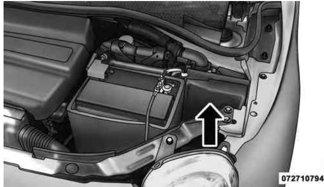
Front Distribution Unit
