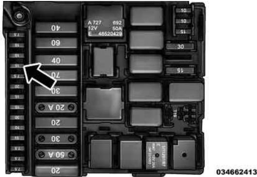
Power Outlet Fuse Location Underhood
