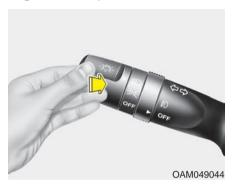
To turn on the high beam headlights, push the lever away from you. Pull it back for low beams.
