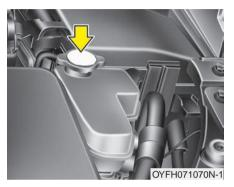
The high-pressure cooling system has a reservoir filled with year-round antifreeze coolant. The reservoir is filled at the factory.
