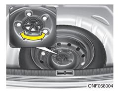
Turn the tire hold-down wing bolt counterclockwise.
