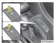
The seat warmers are provided to warm the front seats during cold weather. With the ignition switch in the ON position, push either of the switches to warm the driver's seat or the front passenger's seat.
