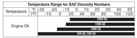
For better fuel economy, it is recommended to use the engine oil of a viscosity grade SAE 5W-20 (API SM / ILSAC GF-4). However, if the engine oil is not available in your country, select the proper engine oil using the engine oil viscosity chart.
