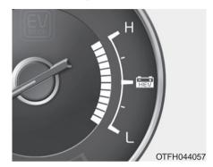
The state of charge (SOC) gauge indicates the hybrid battery's charge level. If the SOC is near L level, the vehicle automatically operates the engine to charge the battery. However, if the service indicator and MIL(Malfunction indicator lamp) turn on when the State of Charge(SOC) is near L(Low), have your vehicle checked by an authorized Kia dealer immediately.
