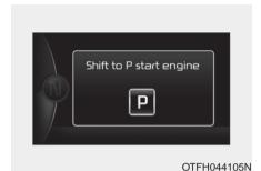
This warning message illuminates if you try to start the engine with the shift lever not in the P (Park) position.
