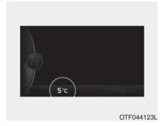
This display indicates the current outside air temperatures by 1°C (1°F).
