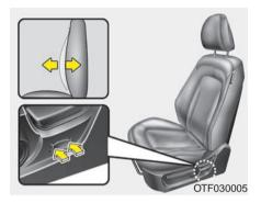
Press the front portion of the switch to increase support, or the rear portion of the switch to decrease support.
