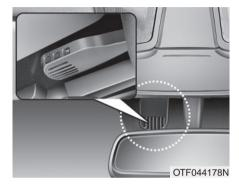
Auto defogging reduces the probability of fogging up the inside of the windshield by automatically sensing the moisture inside the windshield.
