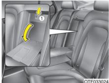
Pull the armrest down using the strap provided on the armrest. Pull the cover down while pushing the release lever down. Additional cargo space is provided to accommodate long/narrow cargo (skis, poles, lumber, etc.) not able to fit properly in the trunk when closed. Make sure the engine is off, the shift lever is in P and the parking brake is applied whenever loading or unloading cargo. The vehicle may move if the shift lever is inadvertently moved to another position.
