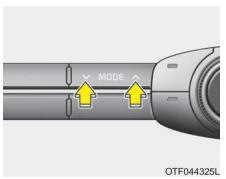
The mode selection button controls the direction of the air flow through
