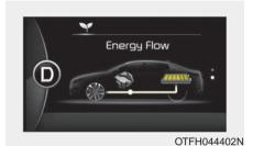
Hybrid battery is being charged by regenerative braking.
