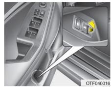
To open the trunk from inside the vehicle, pull the trunk lid release button.
