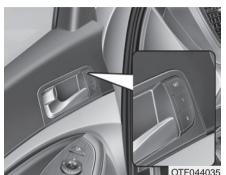
A driver position memory system is provided to store and recall the driver seat position with a simple button operation. By saving the desired position into the system memory, different drivers can reposition the driver seat based upon their driving preference. If the battery is disconnected, the position memory will be lost and the driving position should be restored in the system.
