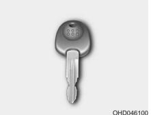
Your vehicle may be equipped with an electronic engine immobilizer system to reduce the risk of unauthorized vehicle use.
