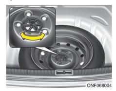
Turn the tire hold-down wing bolt counterclockwise.
