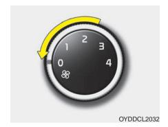
To turn off the blowers, turn the fan speed control knob to the "0" position.
