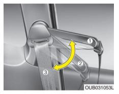
You can adjust the position of the shoulder belt extension guide for easier access to the shoulder belt.
