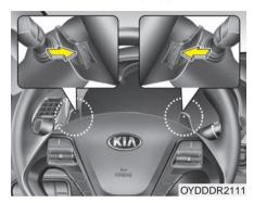
The paddle shifter is available when the shift lever is in the D position or the sport mode.
