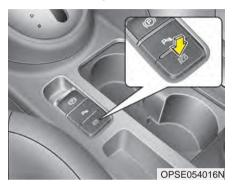
Active ECO helps improve energy efficiency by controlling certain motor and climate contol system operating parameters. Energy efficiency depends on the driver's driving habit and road condition.
