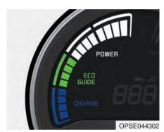
It shows the energy consumption rate of the vehicle and the charge/discharge status of the regenerative brakes.
