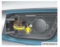
Open the charging door and press the normal charging inlet release tab (1) to open the normal charging inlet cover.
