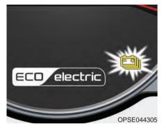
When there are 4 gauge bars (near the "MIN" area) on the high voltage charge indicator, the warning lamp turns ON to alert you of the battery level.
