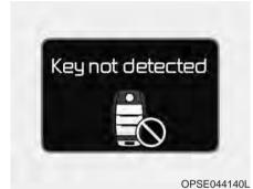
This warning message illuminates if the smart key is not detected when you press the POWER button.
