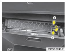
3. Remove the climate control air filter case by pulling out both sides of the cover (1).
