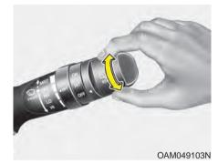
The rear window wiper switch is located at the end of the wiper and washer switch lever. Turn the switch to the desired position to operate the rear wiper and washer.
