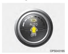
Push the AUTO button. It is indicated by AUTO on the display. The modes, fan speeds, air intake, airconditioning and heater will be controlled automatically by temperature setting.
