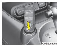
If the battery is weak or the smart key does not work correctly, you can start the vehicle by pressing the POWER button with the smart key.
