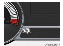
8. Check if the charge indicator lamp of the high voltage battery in the instrument cluster is turned ON. Charging is not done when the charging indicator lamp is OFF.
