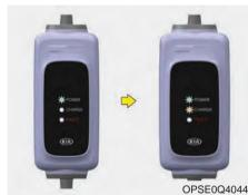
10. Charging starts automatically. Check if the power lamp and charging lamp (orange) are ON.
