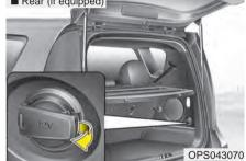
The power outlet is designed to provide power for mobile telephones or other devices designed to operate with vehicle electrical systems.
