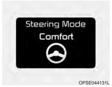
The steering wheel becomes lighter. The comfort mode is usually used when driving in the city or when parking the vehicle.
