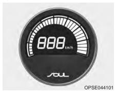
The speedometer indicates the speed of the vehicle and is calibrated in miles per hour (mph) or kilometers per hour (km/h).
