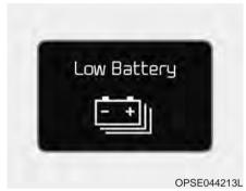
When the high voltage battery level reaches below 20%, this warning message illuminates.
