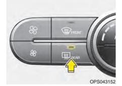
The defroster heats the window to remove frost, fog and thin ice from the rear window, while the vehicle is in the ready ( 2 ) mode.
