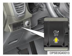
To immediately charge the battery (not at reserved time only) first connect the charging cables. Then, the Deactivate Reserved Charge button [%] should be pressed within three minutes after the cable connection.
