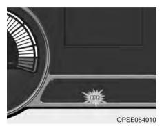
This warning light illuminates if the POWER button is changed to the ON position and goes off in approximately 3 seconds if the system is operation normally.
