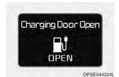
When the vehicle is started while the charging door is opened, this warning message illuminates. Make sure to close the charging door after charging is complete.
