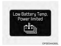
This warning message illuminates to protect battery and electric vehicle system when the high voltage battery temperature is too low.
