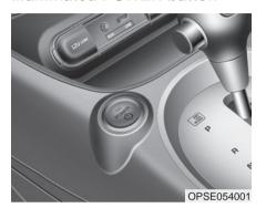
Whenever the front door is opened. the POWER button will illuminate for your convenience. The light will go off after about 30 seconds when the door is closed.
