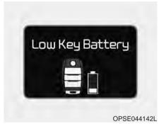
This warning message illuminates if the battery of the smart key is discharged when the POWER button changes to the OFF position.
