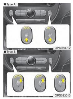
The seat warmer is provided to warm the front seats during cold weather. With the POWER button in the ON position, push either of the switches to warm the driver's seat or the front passenger's seat.
