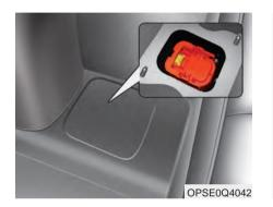
Do not touch the service plug installed at the rear seat footrest. The service plug is designed to block high voltage electricity when repairing the vehicle. If you are careless when handling the service plug, an electric shock may occur.
