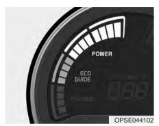
It shows the energy consumption rate of the vehicle and the charge/discharge status of the regenerative brakes.
