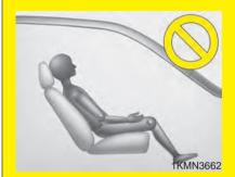
The driver must advise the passenger to keep the seatback in an upright position whenever the vehicle is in motion. If a seat is reclined during an accident, the occupant's hips may slide under the lap portion of the seat belt, applying great force to the unprotected abdomen.
