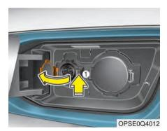
5. Open the charging door and press the normal charging inlet cover release tab (1) to open the normal charging inlet cover.
