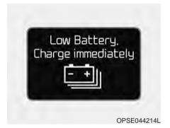
When the high voltage battery level reaches below 10%, this warning message illuminates.
