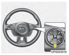
Push the SET - switch, and release it at the desired speed. The SET indicator light in the instrument cluster will illuminate. Release the accelerator pedal at the same time. The desired speed will automatically be maintained.
