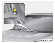
Never place anything over the sensor located on the instrument panel to ensure better control of the heating and cooling system.
