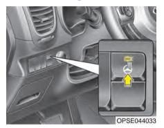
With the POWER button in the ON position, pressing the heated steering wheel button warms the steering wheel. The indicator on the button will illuminate.
