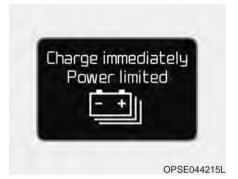
When the high voltage battery level reaches below 7%, this warning message illuminates.
