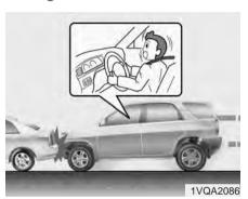
In certain low-speed collisions the air bags may not deploy. The air bags are designed not to deploy in such cases because they may not provide benefits beyond the protection of the seat belts in such collisions.
