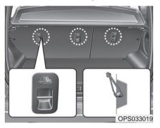
Child restraint hook holders are located on the back of the rear seat-backs.
