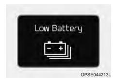
When the high voltage battery level reaches below 20%, this warning message illuminates.
