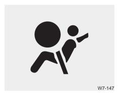
If the air bag warning light illuminated for more than, 6 seconds after the POWER button is turned on, or of it illuminates during vehicle operation, an SRS component may not be functioning properly and you should have your vehicle checked by an authorized Kia dealer.
