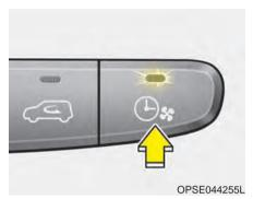
If you press the reserved climate control button (🕒), the indicator lamp inside the button blinks three times and the settings for reserved climate control is displayed on AVN.
