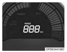
On average, a vehicle can drive about 148km (93miles) when the high voltage battery is 100% charged.
