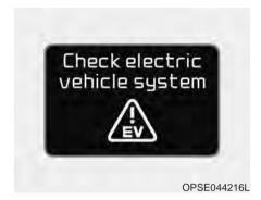
This warning message illuminates when a failure related to EV control system occurs.
