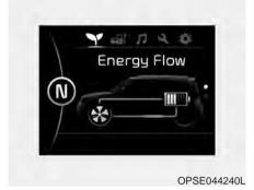
EV energy flow notifies the drivers of energy flow in operating modes. Following modes show drivers the current operating condition.
