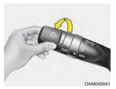
When the light switch is in the parking light position (1st position), the tail, license and instrument panel lights will turn ON.
