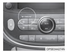
When the POWER button is in the ON position, the clean air function turns on automatically.
