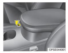
These compartments can be used to store small items required by the driver or front passenger.
