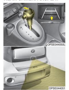
The rear camera display will activate when the back-up light is ON with the POWER button ON and the shift lever in the R (Reverse) position.
