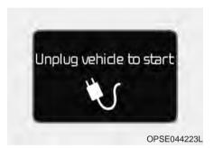
When the vehicle is started while the charging connector is connected, this warning message illuminates.
