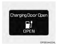
When the vehicle is started while the charging door is opened, this warning message illuminates. Make sure to close the charging door after charging is complete.
