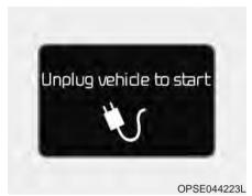
When the vehicle is started while the charging connector is connected, this warning message illuminates.
