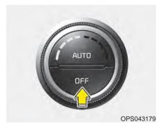
Push the OFF button to turn off the blower. However you can still operate the mode and air intake buttons as long as the POWER button is in the position ON.
