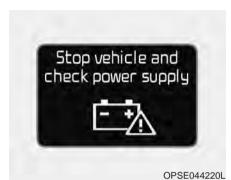
This warning message illuminates when a failure occurs in the power supply system. In this case, park the vehicle in a safe location and tow vour vehicle to the nearest authorized Kia dealer and have the vehicle inspected.
