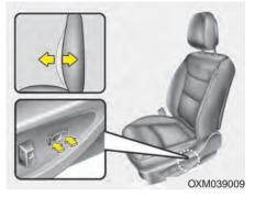
The lumbar support can be adjusted by pressing the button.
