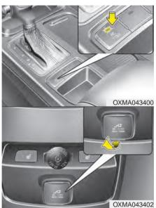
If you press the AC inverter button again, the AC inverter will be deactivated and the light on the AC inverter button will turn off.
