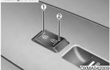
Operate by pressing the central door lock switch.
