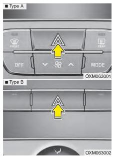
The hazard warning flasher should be used whenever you find it necessary to stop the vehicle in a hazardous location. When you must make such an emergency stop, always pull off the road as far as possible. The hazard warning lights are turned on by pushing in the hazard switch. Both turn signal lights will blink. The hazard warning lights will operate even though the key is not in the ignition switch.
