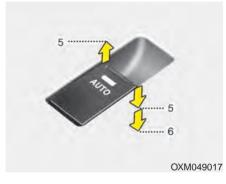
Pressing the power window switch momentarily to the second detent position (6) completely lowers the driver's window even when the switch is released. To stop the window at the desired position while the window is in operation, momentarily pull the switch in the direction opposite of the window's movement.
