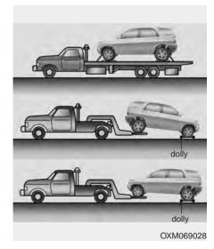
If emergency towing is necessary, we recommend having it done by an authorized Kia dealer or a commercial tow-truck service. Proper lifting and towing procedures are necessary to prevent damage to the vehicle. The use of wheel dollies or flatbed is recommended. For trailer towing guidelines information, refer to "Trailer towing" in section 5.
