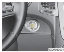
Whenever the front door is opened, the ENGINE START/STOP button will illuminate for your convenience. The light will go off after about 30 seconds when the door is closed. It will also go off immediately when the theft-alarm system is armed. ENGINE START/STOP button position
