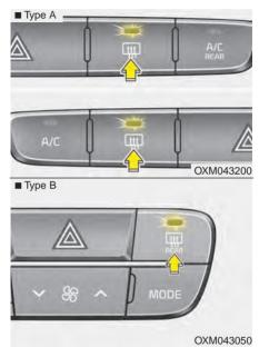
The defroster heats the window to remove frost, fog and thin ice from the rear window, while the engine is running. To activate the rear window defroster, press the rear window defroster button located in the center facia switch panel. The indicator on the rear window defroster button illuminates when the defroster is ON.
