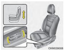
Pull the front portion of the control switch up to raise or press down to lower the front part of the seat cushion. Pull the rear portion of the control switch up to raise or press down to lower the rear part of the seat cushion. Release the switch once the seat reaches the desired position.
