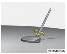
Your vehicle uses a roof antenna to receive AM or/and FM broadcast signals.
