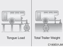
What is the maximum safe weight of a trailer? It should never weigh more than the maximum trailer weight with trailer brakes. But even that can be too heavy.
