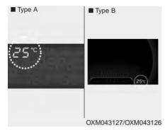
The current outside temperature is displayed in 1°C (1°F) increments. The temperature range is between --40°C ~ 60°C (40°F ~ 140°F).
