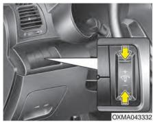
The brightness of the instrument panel illumination is changed by pressing the illumination control button ("+" or "-") when the ignition switch or Engine Start/Stop button is ON, or the tale lights are turned on. Type A
