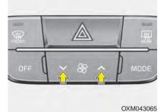
The fan speed can be set to the desired speed by operating the fan speed control switch.
