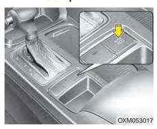
Active ECO helps improve fuel efficiency by controlling certain engine and transaxle system operating parameters. Fuel efficiency depends on the driver's driving habit and road condition.
