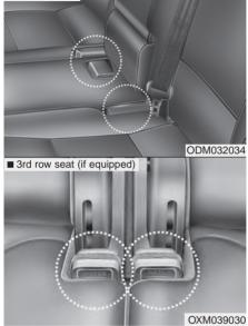
The rear seat belt buckles can be stowed in the pocket between the rear seatback and cushion when not in use. 2nd row seat
