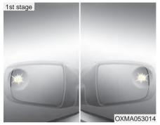
If a vehicle is detected within the boundary of the system, a yellow warning light will illuminate inside of the outside rearview mirror glass.
