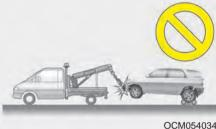
Failure to place the transaxle shift lever in N (Neutral) may cause internal damage to the transaxle.
