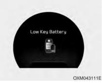
• This warning message illuminates if the battery of the smart key is discharged when the Engine Start/Stop Button changes to the OFF position. Press start button while turn steering (for smart key system)
