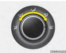
The mode selection knob controls the direction of the air flow through
