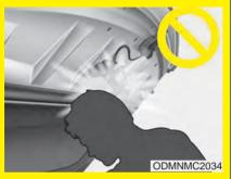
When you check the engine compartment, Take caution to avoid contacting your head with the safety hook which is located inside of the hood.
