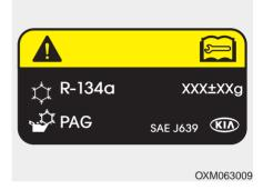
The actual Air Conditioning refrigerant label in the vehicle may differ from the illustration. Each symbols and specification on air conditioning refrigerant label means as below ;
