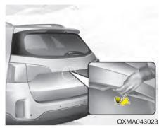
• Press the tailgate handle switch carrying the smart key with you.
