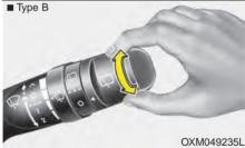
The rear window wiper and washer switch is located at the end of the wiper and washer switch lever. Turn the switch to the desired position to operate the rear wiper and washer.
