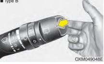
In the OFF position, pull the lever gently toward you to spray washer fluid on the windshield and to run the wipers 1-3 cycles.
