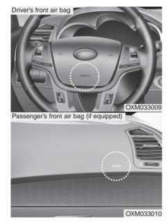
Your vehicle is equipped with an Advanced Supplemental Restraint (Air Bag) System and lap/shoulder belts at both the driver and passenger seating position. The indication of the system's presence are the letters "AIR BAG" embossed on the air bag pad cover on the steering wheel and the passenger's side front panel pad above the glove box.
