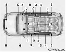
The SRS consists of the following components:
