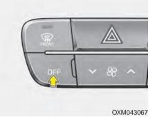
Press the front blower OFF button to turn off the front air climate control system. However, you can still operate the mode and air intake buttons as long as the ignition switch is in the ON position. Climate information screen selection (for Type C, D)
