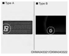
This indicator displays which automatic transaxle shift lever is selected.
