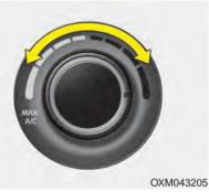
The temperature control knob allows you to control the temperature of the air flowing from the ventilation system. To change the air temperature in the passenger compartment, turn the knob to the right position for warm and hot air or left position for cooler air.
