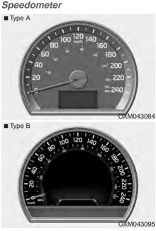
The speedometer indicates the speed of the vehicle and is calibrated in kilometers per hour (km/h) and/or miles per hour (mph).
