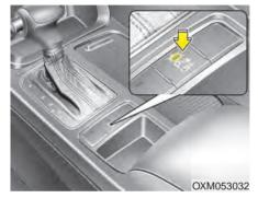
• This system will activate when the indicator on the rear parking assist OFF button is not illuminated. If you desire to deactivate the rear parking assist system, press the rear parking assist OFF button again. (The indicator on the button will illuminate.) To turn the system on, press the button again. (The indicator on the button will go off.)
