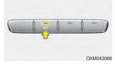
Press the A/C button to turn the air conditioning system on (indicator light will illuminate).
