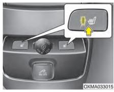
The seat warmer is provided to warm the rear seats during cold weather. With the ignition switch in the ON position, push either of the switches to warm rear seats.
