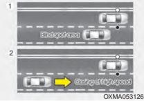
The BSD (Blind spot detection) system uses a radar sensor to alert the driver while driving.
