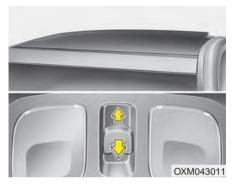
Before opening or closing the sunroof, open the roller blind (refer to the following page for instructions on how to use the roller blind).
