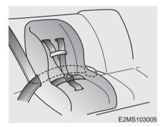
The auto lock mode will help prevent the normal movement of the child in the vehicle from causing the seat belt to loosen and compromise the child restraint system. To secure a child restraint system, use the following procedure.
