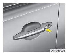
Pressing the button of the front outside door handles with all doors closed and any door unlocked, locks all the doors. The hazard warning lights will blink and the chime will sound once to indicate that all doors are locked. The button will only operate when the smart key is within 0.7~1 m (28~40 in.) from the outside door handle. If you want to make sure that a door has locked or not, you should check the door lock button inside the vehicle or pull the outside door handle.
