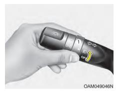
Fog lights are used to provide improved visibility when visibility is poor due to fog, rain or snow, etc. The fog lights will turn on when the fog light switch (1) is turned to the on position after the headlights are turned on.
