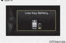
This warning message illuminates if the battery of the smart key is discharged when the Engine Start/Stop Button changes to the OFF position.
