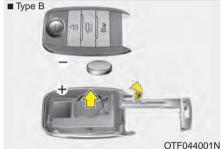
A battery should last for several years, but if the transmitter or smart key is not working properly, try replacing the battery with a new one. If you are unsure how to use or replace the battery, contact an authorized Kia dealer.
