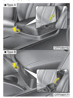
To open the center console storage, pull the lever up.
