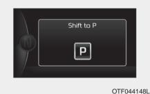
This warning message illuminates if you try to turn off the engine without the shift lever in P (Park) position.  At this time, the Engine Start/Stop Button turns to the ACC position (If you press the Engine Start/Stop Button once more, it will turn to the ON position).
