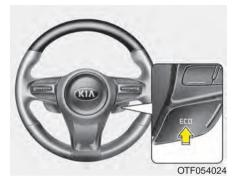
Active ECO helps improve fuel efficiency by controlling the engine and transaxle. But fuel-efficiency can be affected by the driver's driving habits and road conditions.
