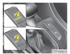
The air ventilation is provided to cool the driver's seat during hot weather by blowing air through small vent holes on the surface of the seat and seatback. While the engine is running, press the switch to cool the seat.
