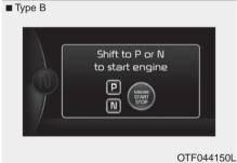
This warning message illuminates if you try to start the engine with the shift lever not in the P (Park) or N (Neutral) position.
