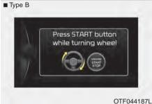
This warning message illuminates if the steering wheel does not unlock normally when the Engine Start/Stop Button is pressed.  It means that you should press the Engine Start/Stop Button while turning the steering wheel right and left.
