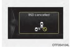
The message will appear to notify the driver if there are foreign substances on the rear bumper or it is hot near the rear bumper. The light on the switch and the system will turn off automatically. Remove the foreign matter on the rear bumper.
