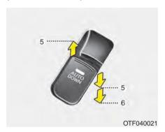
Pressing the power window switch momentarily to the second detent position (6) completely lowers the driver's window even when the switch is released. To stop the window at the desired position while the window is in operation, momentarily pull up the switch to the opposite direction of the window movement.
