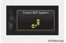
If the system does not work properly, a warning message will appear and the light on the switch will turn off. The
