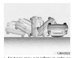
Air bags may not inflate in rollover accidents because the vehicle can not detect rollover accident.
