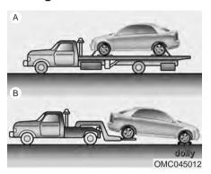
If emergency towing is necessary, we recommend having it done by an authorized Kia dealer or a commercial tow-truck service. Proper lifting and towing procedures are necessary to prevent damage to the vehicle. The use of wheel dollies or flatbed is recommended.
