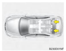
Some child seat manufacturers make child restraint seats that are labeled as LATCH or LATCH-compatible child restraint seats. LATCH stands for "Lower Anchors and Tethers for Children". These seats include two rigid or webbing mounted attachments that connect to two LATCH anchors at specific seating positions in your vehicle. This type of child restraint seat eliminates the need to use seat belts to attach the child seat in the rear seats.
