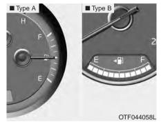
The fuel gauge indicates the approximate amount of fuel remaining in the fuel tank. The fuel tank capacity is given in chapter 8. The fuel gauge is supplemented by a low fuel warning light, which will illuminate when the fuel tank is nearly empty.
