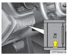
The Electronic Stability control (ESC) system is designed to stabilize the vehicle during cornering maneuvers. ESC checks where you are steering and where the vehicle is actually going. ESC applies the brakes on individual wheels and intervenes with the engine management system to stabilize the vehicle. Electronic stability control (ESC) will
