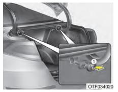
Pull the lock release lever (1) and fold the rear seatback forward and down firmly.
