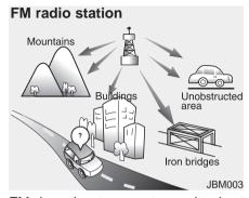
FM broadcasts are transmitted at high frequencies and do not bend to follow the earth's surface. Because of this, FM broadcasts generally begin to fade within short distances from the station. Also, FM signals are easily affected by buildings, mountains, and obstructions. This can lead to undesirable or unpleasant listening conditions which might lead you to believe a problem exists with your radio. The following conditions are normal and do not indicate radio trouble:
