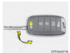
To unfold the key, press the release button and the key will unfold automatically.
