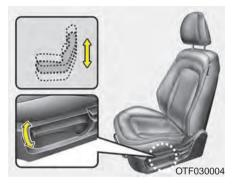
To change the height of the seat cushion push the lever upwards or downwards.
