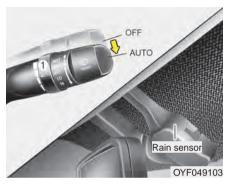
The rain sensor located on the upper end of the windshield glass senses the amount of rainfall and controls the wiping cycle for the proper interval. The more it rains, the faster the wiper operates. When the rain stops, the wiper stops. To vary the speed setting, turn the speed control knob (1).
