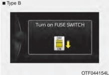
This warning message illuminates if the fuse switch on the fuse box is OFF. • It means that you should turn the fuse switch on.
