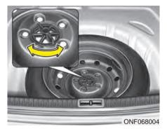
Turn the tire hold-down wing bolt counterclockwise.
