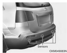
The rear parking assist system assists the driver during backward movement of the vehicle by chiming if any object is sensed within a distance of 47 in. (120 cm) behind the vehicle.
