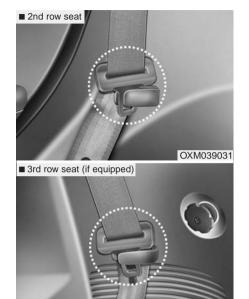
Routing the seat belt webbing through the rear seat belt guides will help keep the belts from being trapped behind or under the seats.
