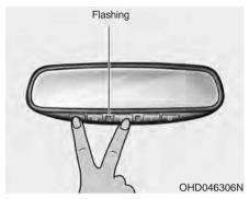
1. When programming the buttons for the first time, press and hold the left and center buttons ( ①, ①) simultaneously until the indicator light begins to flash after approximately 20 seconds. (This procedure erases the factory-set default codes. Do not perform this step when programming the additional HomeLink buttons.)
