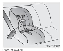
Placing a passenger seat belt into the auto lock mode
