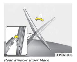
Raise the wiper arm and pull out the wiper blade assembly.
