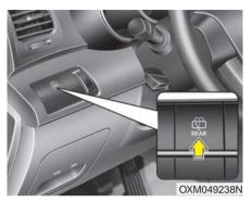
Press the button to spray rear washer fluid and to run the rear wipers.
