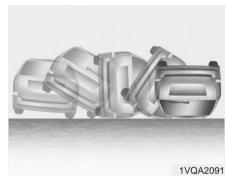
Front air bags may not inflate in all rollover accidents where the SRSCM indicates that the SRSCM indicates that the front air bag deployment would not provide additional occupant protection.
