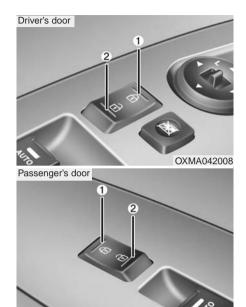
D050202AAM-FU With central door lock switch Operate by pressing the central door lock switch.
