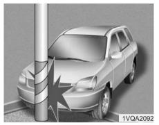
Air bags may not inflate if the vehicle collides with objects such as utility poles or trees, where the point of impact is concentrated to one area and the full force of the impact is not delivered to the sensors C041100AUN
