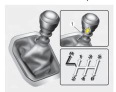
The shift lever can be moved without pulling the ring (1).
