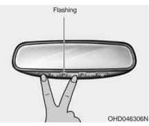
When programming the buttons for the first time, press and hold the left and center buttons (①, ①) simultaneously until the indicator light begins to flash after approximately 20 seconds. (This procedure erases the factory-set default codes. Do not perform this step when programming the additional HomeLink buttons.)
