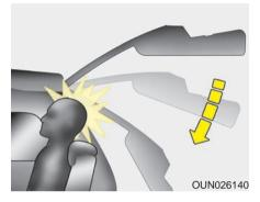
WARNING - 3rd row seat 3rd row occupants should always remain in the center of the seat cushion so the occupants head is protected by the headrest. If not, the tailgate may hit the occu-
