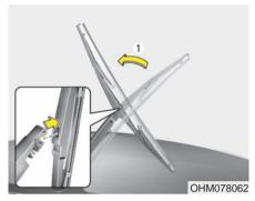
*Rear window wiper blade* 1. Raise the wiper arm and pull out the wiper blade assembly.
