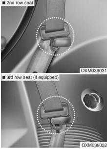
Routing the seat belt webbing through the rear seat belt guides will help keep the belts from being trapped behind or under the seats.
