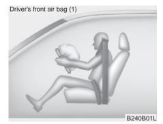
The front air bag modules are located both in the center of the steering wheel and in the front passenger's panel above the glove box. When the SRSCM detects a sufficiently severe impact to the front of the vehicle, it will automatically deploy the front air bags. Driver's front air bag (2)
