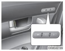
A driver position memory system is provided to store and recall the driver's seat, outside rearview mirror and steering wheel position or the instrument panel illumination intensity with a simple button operation. By saving the desired positions into the system memory, different drivers can reposition the positions based upon their driving preference. If the battery is disconnected, the position memory will be erased.
