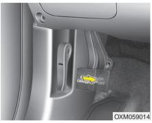
*Releasing the parking brake* Foot type
