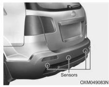
The rear parking assist system is a supplementary function only. The operation of the rear parking assist system can be affected by several factors (including environmental conditions). It is the responsibility of the driver to always check the area behind the vehicle before and while backing up.
