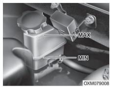
If the level is low, add fluid to the MAX level. The level will fall with accumulated mileage. This is a normal condition associated with the wear of the brake linings and/or clutch disc (if equipped). If the fluid level is excessively low, have the brake/clutch\* system checked by an authorized KIA dealer.
