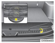
3. Use the wheel lug nut wrench to loosen the bolt enough to lower the spare tire.
