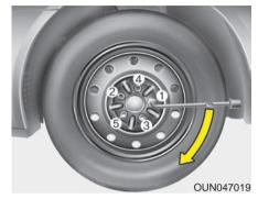
Then position the wrench as shown in the drawing and tighten the wheel nuts. Be sure the socket is seated completely over the nut. Do not stand on the wrench handle or use an extension pipe over the wrench handle. Go around the wheel tightening every nut following the numerical sequence shown in the image until they are all tight. Then double-check each nut for tightness. After changing wheels, have an authorized KIA dealer tighten the wheel nuts to their proper torque as soon as possible.
