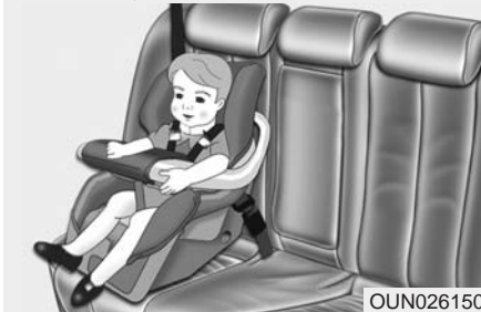
Forward-facing child restraint system
