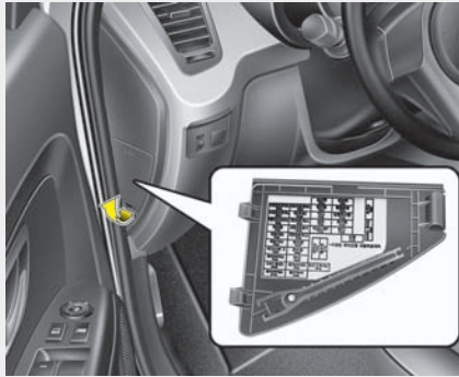
Inner fuse panel
