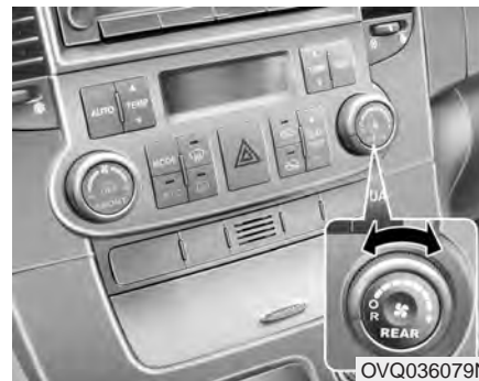
Rear fan speed control
