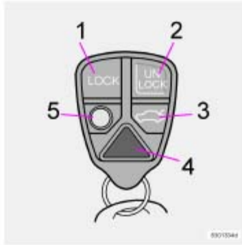
Buttons in remote control: 1 - Lock, 2 - Unlock, 3 - Open trunk, 4 - "Panic" function*, 5 - Approach lighting
