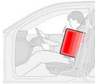
The SIPS airbag system is designed to help increase occupant protection in the event of certain side impact collisions. The SIPS airbags are designed to deploy only during certain side-impact collisions, depending on the crash severity, angle, speed and point of impact. SIPS airbag deployment (one airbag) occurs only on the side of the vehicle affected by the impact. The airbags are not designed to deploy in all side impact situations.
