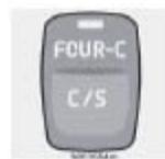
Use the button in the center console to switch between the driving modes Comfort and Sport. This can be done at any time.
