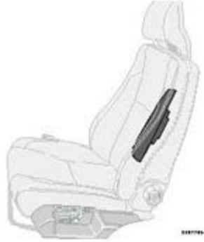
Location of the side impact (SIPS) airbag
