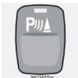
The system is always activated when the car is started. Press the button to deactivate/reactivate the parking assistance system. See also page 125.
