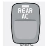
Press the button to activate the air conditioning in the rear of the passenger compartment. Rear air conditioning is deactivated when the ignition is completely switched off.
