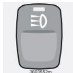
Use this button to switch the auxiliary lamps on with main beam or to switch them off. The LED in the button is lit when the function is activated.
