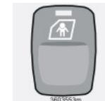
Use this button to activate or deactivate the electric child safety locks in the rear doors. The ignition key must be in position **I** or **II**. When the child safety locks are activated, the LED in the button lights. A message is shown on the display when the child safety locks are activated or deactivated.
