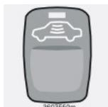
Use this button when you wish to switch off the deadlock function (doors cannot be opened from the inside when locked). This button can also be used
