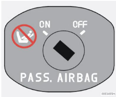
*Switch for SRS in ON position.*
