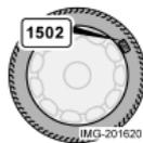
Tyres are perishable. After a few years they begin to harden at the same time as the friction capacity/characteristics gradually deteriorate. Therefore aim to get as fresh tyres as possible when you replace them. This is especially important with regard to winter tyres. The week and year of manufacture, the tyre's DOT marking (Department of Transportation), are stated with four digits, for example 1502. The tyre in
