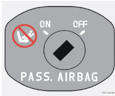
*Switch for SRS in OFF position.*
