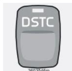
This button is used to reduce or reactivate the functions of the DSTC system. When the LED in the button is lit, the DSTC system is activated (assuming there is no fault).
