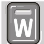
The **W** button by the gear selector engages and disengages the winter programme **W**. The symbol **W** is shown in the combined instrument panel when the winter programme is activated.
