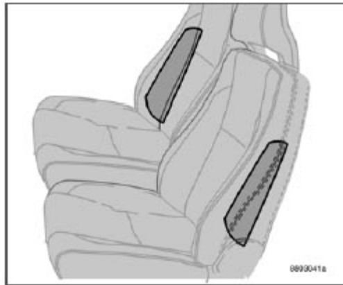
Location of the side impact (SIPS) airbag
