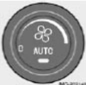
The blower speed can be increased or decreased by turning the knob. The blower speed is regulated
