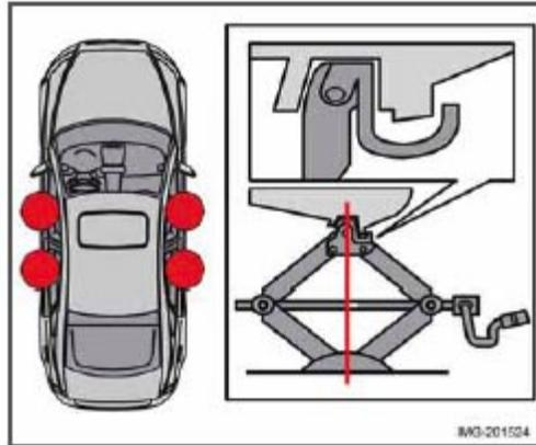
7. Raise the vehicle until the wheel to be changed is lifted off the ground.
