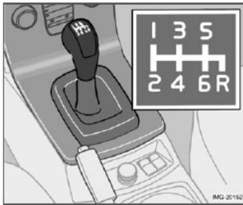
Depress the clutch pedal completely when changing gears<sup>1</sup>.
