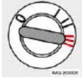
Turn the key to this position and release it immediately. The key returns automatically to the Drive position. A chime will sound if the key is left in the ignition and the driver's door is opened (does not apply to vehicles with the optional keyless drive).
