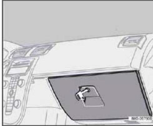
The owners manual and maps can be stored here. There are also holders for coins, pens and fuel cards. The glove compartment can only be locked and unlocked using the detachable key blade from the central locking system's remote control. See the chapter "Locks and alarm" for further information about the key blade.
