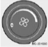
The blower speed can be increased or decreased by turning the knob. If the knob is turned counterclockwise and the indicator light in the display goes out, the blower and the air conditioning are switched off. The display shows the blower symbol and OFF.
