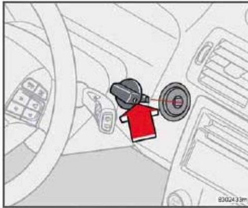
Removing the keyless drive start control
