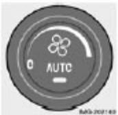
The AUTO function automatically regulates climate control to maintain the desired temperature. The automatic function controls heating, air conditioning, blower speed, recirculation, and air distribution.
