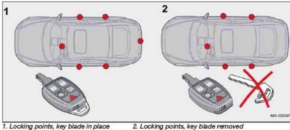
By utilizing the remote control with the key blade removed, the valet locking feature enables you to block access to the trunk and glove compartment for e.g. valet parking or when the car is brought to the retailer for service.
