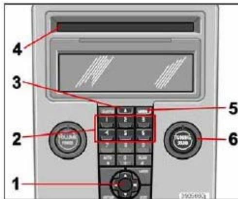
1. **MENU NAVIGATION CONTROL**-press the up or down arrow keys to scroll in a menu, or the keys on the left/right sides of the control to change CD tracks/fast forward/back
