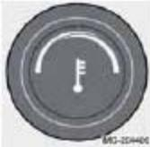
The knob with the thermometer symbol is used to select cooling or heating for both the driver's and passenger's sides of the car.
