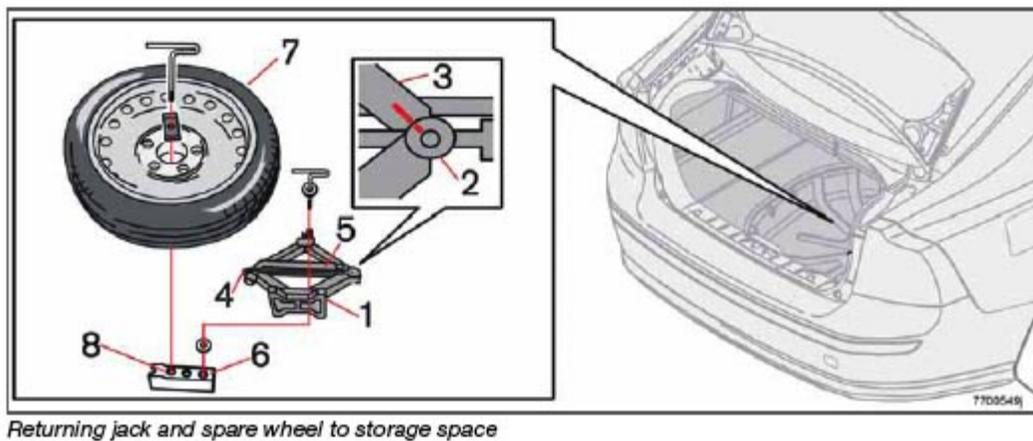
1. Crank the jack (1) down approximately halfway until the mark on the washer (2) aligns with the mark on the jack's arm (3).
