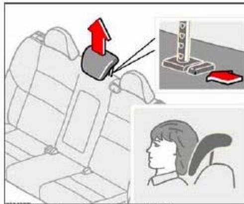
*Adjust the head restraint vertically*
