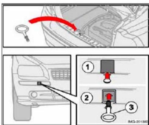
The towing eyelet is located under the floor of the cargo area. This eyelet must be screwed into the positions provided on the right sides of either the front or rear bumper (see illustrations).
