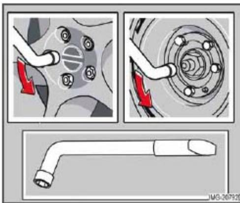
5. With the car still on the ground, use the lug wrench to loosen the wheel nuts 1/2 - 1 turn by exerting downward pressure. Turn the nuts counterclockwise to loosen.
