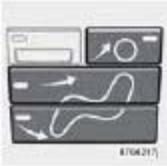
Press one of the three buttons in the illustration to activate the selected airflow. A symbol in the display above the climate control panel and a lit LED in the selected button indicate that the manual function has been selected. With manually selected airflow both warm and cool air can be selected. The desired temperature is selected using control 9.
