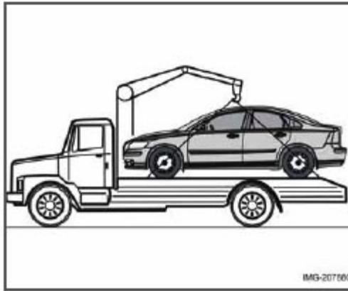
Volvo recommends the use of flat bed equipment for towing vehicles with front wheel drive. If wheel lift equipment must be used, please use extreme caution to help avoid damage to the vehicle.
