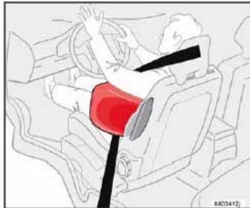
Components in the SIPS airbag system
