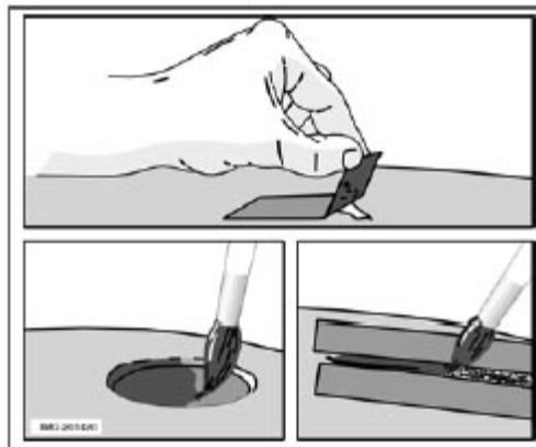
1. Place a strip of masking tape over the damaged surface. Pull the tape off so that any loose flakes of paint adhere to it.
