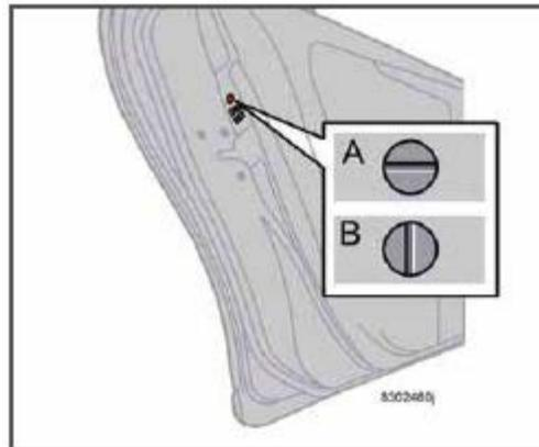
The controls are located on the rear inside edges of the doors, and are only accessible when the doors are open. Use the ignition key blade or a screwdriver to turn the control.
