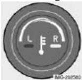
The temperatures on the driver's and passenger's sides can be set separately using the knob (with the thermometer in it). The temperature can be set for both sides of the car when the ignition is switched on (both LEDs will be on), which means that a temperature setting will apply to both sides of the car.
