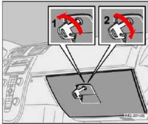
The glove compartment can only be locked and unlocked using the detachable key blade on the remote control. See [page 109](#) for information on removing the key blade from the remote control.
