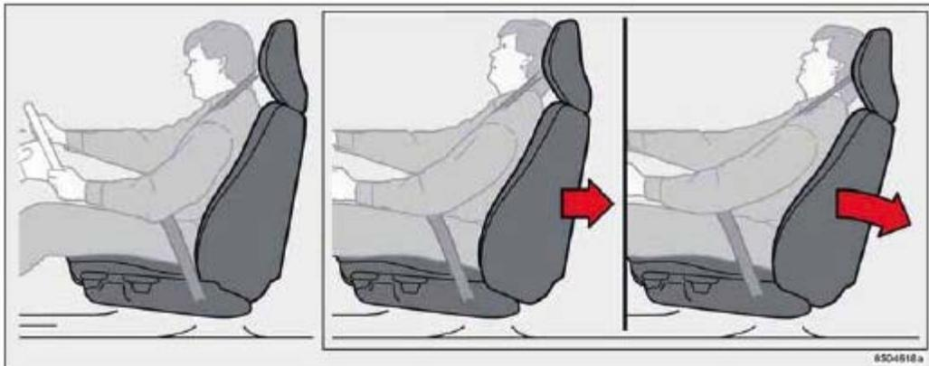
The WHIPS system consists of specially designed hinges and brackets on the front seat backrests designed to help absorb some of the energy generated in a collision from the rear (when the vehicle is "rear-ended").
