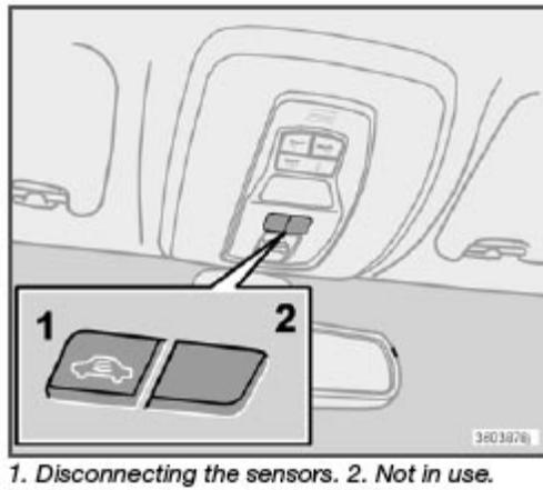
In certain situations it may be desirable to turn off the accessory inclination and movement alarm sensors if, for example, you drive your vehicle onto a ferry where the rocking of the boat could trigger the alarm or if a pet is left in the vehicle with the doors locked.
