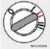
The key's position when driving. The vehicle's entire electrical system is activated.
