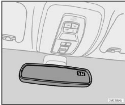
The upper right-hand corner of the rearview mirror has an integrated display that shows the compass direction toward which the car is pointing. Eight different directions can be displayed: N, NE, E, SE, S, SW, W and NW. The display shows your car's orientation with respect to true north.
