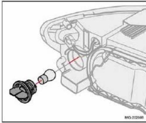
1. Turn the bulb holder counterclockwise and remove it.
