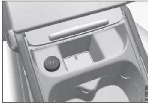
12-volt socket in the front tunnel console
