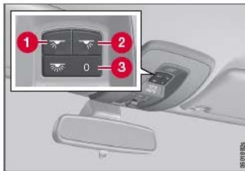
Light switches, front roof lighting
