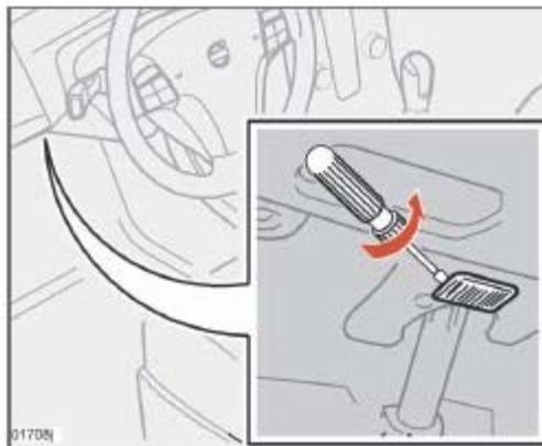
The footwell lighting is located under the dashboard on the driver's and passenger's sides. To replace a bulb:
