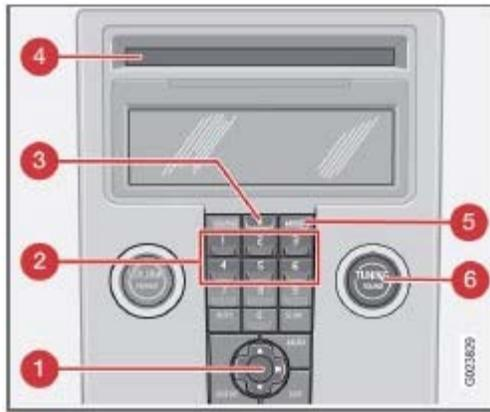
1. **MENU NAVIGATION CONTROL**-press the up or down arrow keys to scroll in a menu, or the keys on the left/right sides of the control to change CD tracks/fast forward/back
