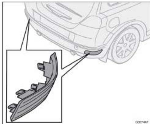
The grids are held in place by clips and can be pressed into position. They can only be installed one way.
