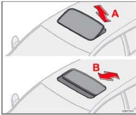
To operate the moonroof, the ignition key must first be turned to the intermediate or drive position (position I, II or the engine running). The moonroof can be opened in two ways:
