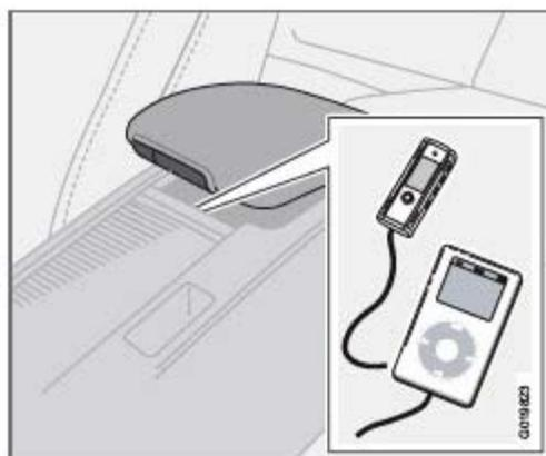
An auxiliary device, such as an iPod or a USB flash drive can be connected to the audio system via the connector in the center console storage compartment.
