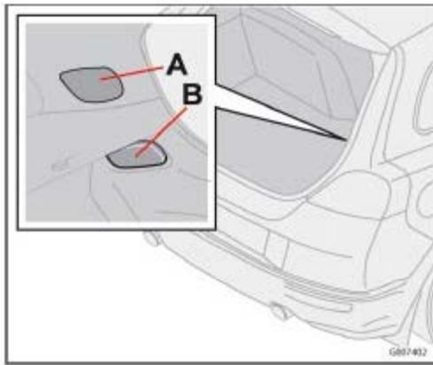
All bulbs in the taillight cluster can be replaced from the cargo area. To access the bulb holders:
