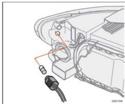
1. Turn the bulb holder counterclockwise, pull it out, and replace the bulb.
