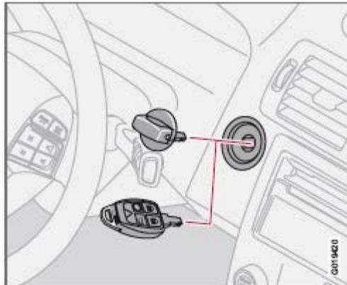
Removing the keyless drive start control
