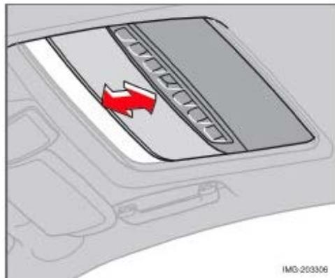
The optional moonroof features a sliding visor. The visor slides open automatically when the moonroof is opened, and
