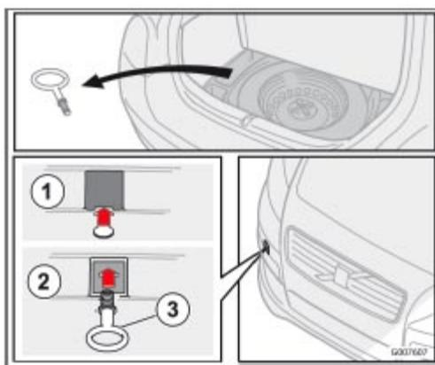
The towing eyelet is located under the floor of the cargo area. This eyelet must be screwed into the positions provided on the right sides of either the front or rear bumper (see illustrations).
