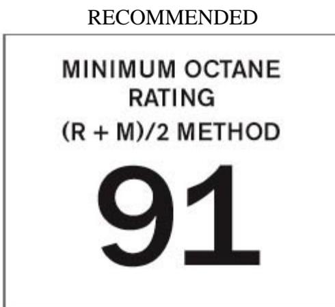
In demanding driving conditions, such as operating the vehicle in hot weather, towing a trailer, or driving for extended periods at higher altitudes than normal, it may be advisable to switch to higher octane fuel (91 or higher) or to change gasoline brands to fully utilize your engine's capacity, and for the smoothest possible operation.
