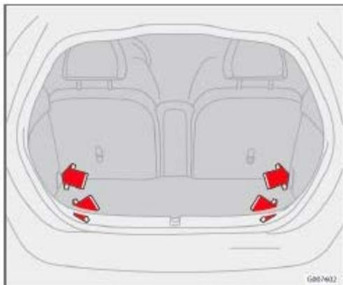
The eyelets in the cargo area can be used to fasten accessory load nets and lashing straps, load nets, and other load anchors.
