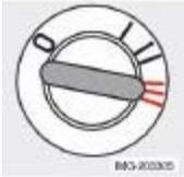
Turn the key to this position and release it immediately. The key returns automatically to the Drive position.
