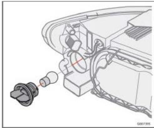
1. Turn the bulb holder counterclockwise and remove it.
