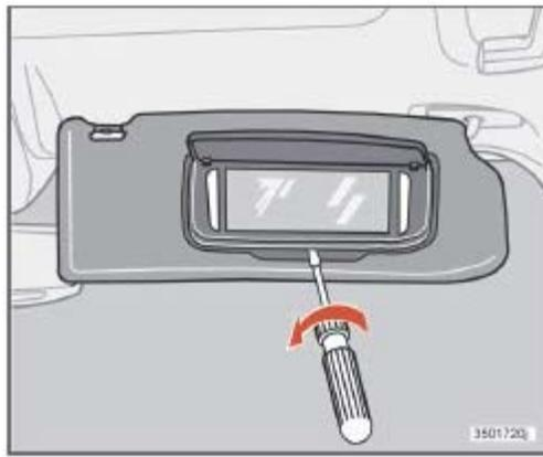
1. Insert a screwdriver under the center of the lower edge of the mirror, turn it, and carefully pry up the lugs at the edge.
