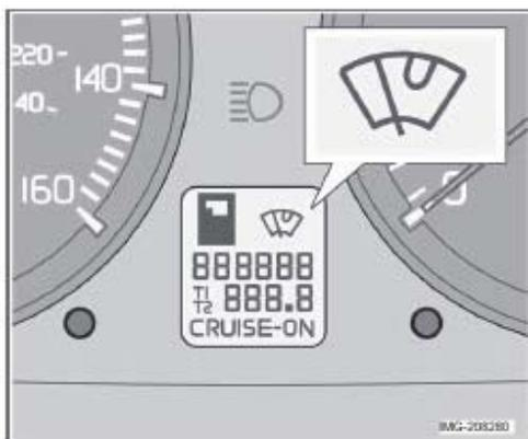
The rain sensor automatically regulates windshield wiper speed according to the amount of water on the windshield. The sensitivity of the rain sensor is adjusted by moving the thumb wheel (C in the illustration on the previous page) up (the wipers will sweep the windshield more frequently) or down (the wipers will sweep the windshield less frequently).
