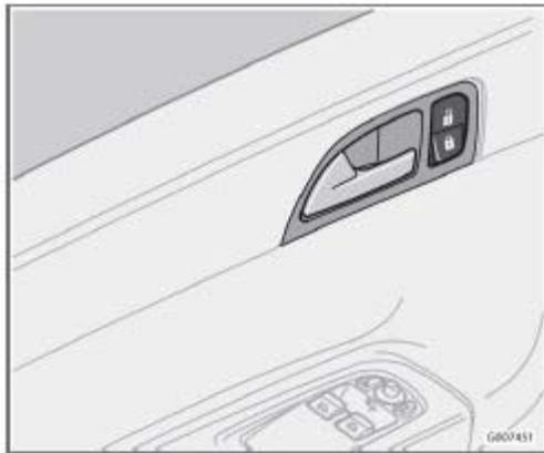
The switches near the door opening handles on the driver's and passenger's doors can be used to lock or unlock both doors and the rear liftgate, open or close the side windows<sup>1</sup>, and to set the alarm.
