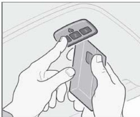
HomeLink<sup>1</sup> is an optional system that can be programmed to learn the codes of three different remote controlled-devices (for example, a garage door opener, remote lighting, entry gate). HomeLink's sun visor-mounted transceiver, powered by your car's electrical system, may then be used in place of your hand-held remote controls. The HomeLink transceiver consists of three programmable buttons and an indicator light.
