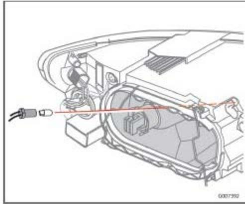
1. Pull out the bulb holder with a pair of pliers. The bulb holder should not be pulled out by the wire.
