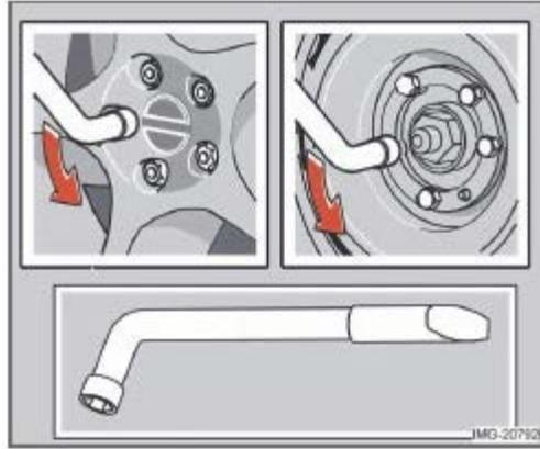
5. With the vehicle still on the ground, use the lug wrench to loosen the wheel nuts 1/2 - 1 turn by exerting downward pressure. Turn the nuts counterclockwise to loosen.
