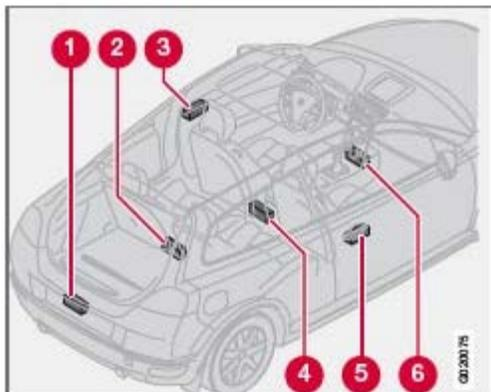
The keyless drive system has a number of antennas located at various points in the vehicle.
