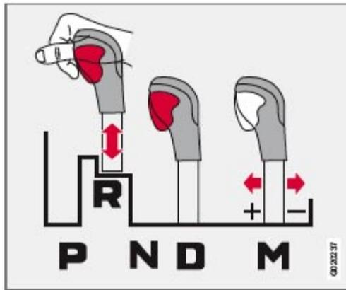
Depress the button on the front of the gear selector knob to move the selector between the R, N, D, and P positions. The gear selector can be moved freely between the Geartronic (manual shifting) and (D)rive positions while driving.
