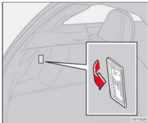
1. Insert a screwdriver and turn it carefully to release the lens.
