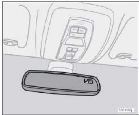
The upper right-hand corner of the rearview mirror has an integrated display that shows the compass direction toward which the vehicle is pointing. Eight different directions can be displayed: N, NE, E, SE, S, SW, W and NW. The display shows your car's orientation with respect to true north.
