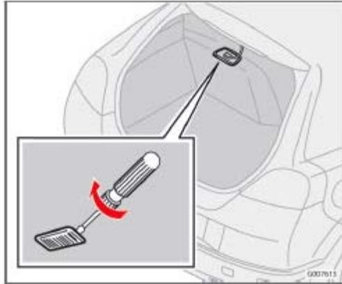
1. Insert a screwdriver and turn it gently to detach the bulb housing.
