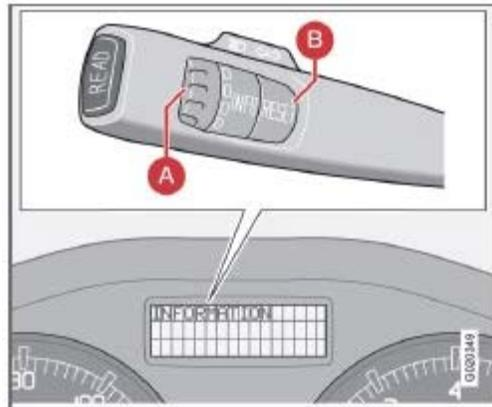
Controls on the left-side steering wheel lever
