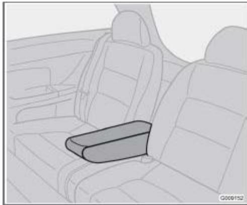
The center armrest can be folded down for comfort or to make room for long objects. The armrest folds down automatically when one of the backrests is folded down.
