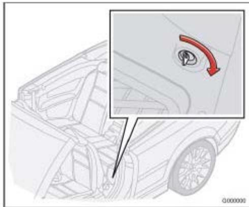
1. Fold down the driver's seat backrest to access the keyhole near the floor of the rear seat.
