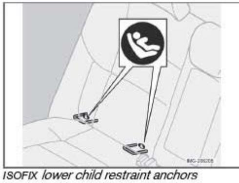
Lower anchors for ISOFIX-equipped child seats are located in both rear seating positions, hidden below the backrest cushions. Symbols on the seat back upholstery mark the anchor positions (see the illustration).
