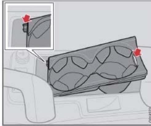
Two cup holders are located under the sliding cover in the center console.
