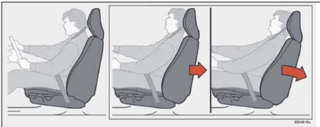
The WHIPS system consists of specially designed hinges and brackets on the front seat backrests designed to help absorb some of the energy generated in a collision from the rear (when the vehicle is "rear-ended").
