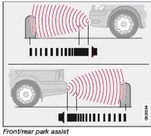
The park assist system is designed to assist you when driving into parking spaces, garages, etc. It utilizes four ultrasound sensors located in one or both bumpers to measure the distance to a vehicle, object, or a person who may be close to the front or rear of your vehicle.
