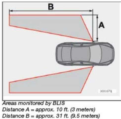
BLIS has an integrated function that alerts the driver if a fault should occur with the system. For example, if one or both of the system's cameras are obscured, a message (see the table on [page 162](#)) will appear in the information display in the instrument panel. If this occurs, clean the camera lenses. If necessary, the system can be temporarily switched off (for instructions, see [page 162](#)).
