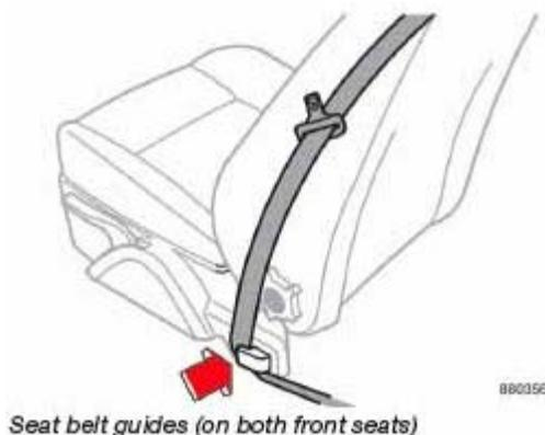
These guides are designed to help provide easier access to the seat belts. A belt can be taken out of the guide and slid to the rearmost part of the lower seat belt anchorage rod to make it easier for passengers to enter or exit the rear seat.
