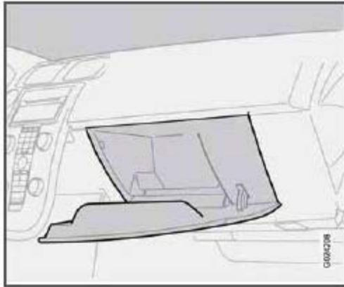
The owners manual and maps can be stored here. There are also holders for coins, pens and fuel cards. The glove compartment can only be locked and unlocked using the detachable key blade from the central locking system's remote control. See [page 115](#) for information on removing the key blade from the remote control, and [page 124](#) for information on locking the glove compartment
