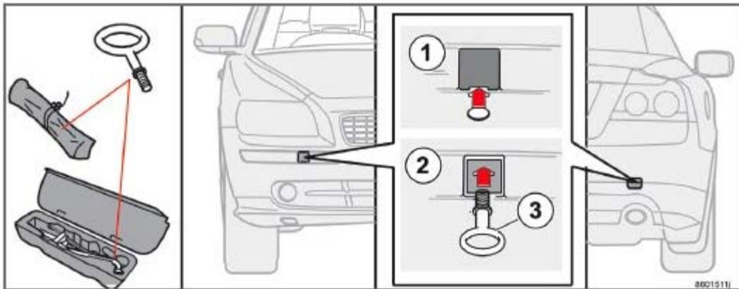
The towing eyelet is located under the floor of the cargo area with the optional temporary spare tire or in the bag stowed in the ski hatch. This eyelet must be screwed into the positions provided on the right sides of either the front or rear bumper (see illustrations).
