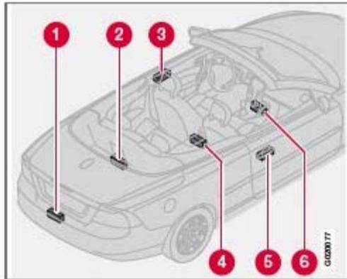
The keyless drive system has a number of antennas located at various points in the vehicle.
