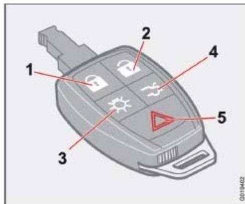
1. **Lock** - Press the Lock button on the remote once to lock both doors, the trunk, the cabin storage compartments (compartment in the doors, the rear side panels, and the ski hatch in the center of the rear seat backrest). The turn signals will flash twice to confirm locking.
