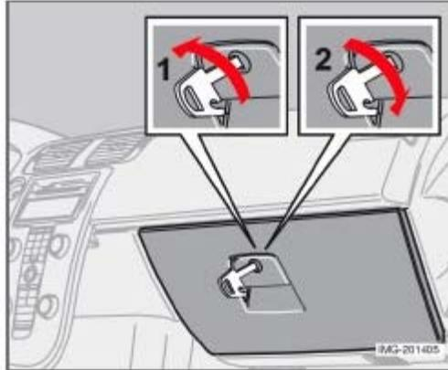
The glove compartment can only be locked and unlocked using the detachable key blade on the remote control. See [page 115](#) for information on removing the key blade from the remote control.
