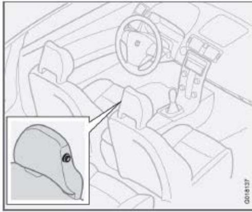
The jacket hanger is located on the inboard side of the front passenger's seat head restraint. It is only intended for hanging light garments.
