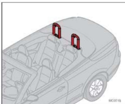
Deployed ROPS roll bars
