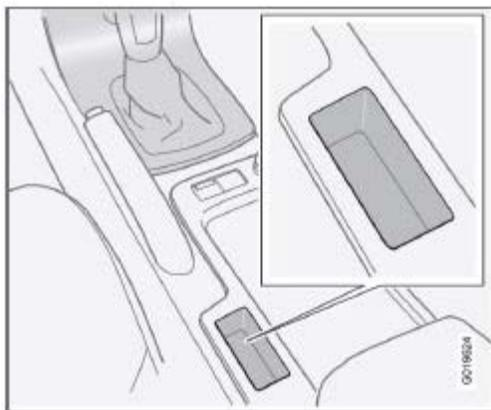
If the buttons for optional equipment are not installed, the recess behind the parking brake can be used as a storage compartment.
