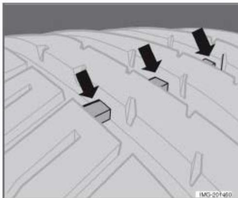
The tires have wear indicator strips running across or parallel to the tread. The letters TWI are printed on the side of the tire. When approximately 1/16" (1.6 mm) is left on the tread, these strips become visible and indicate that the tire should be replaced. Tires with less than 1/16" (1.6 mm) tread offer very poor traction.
