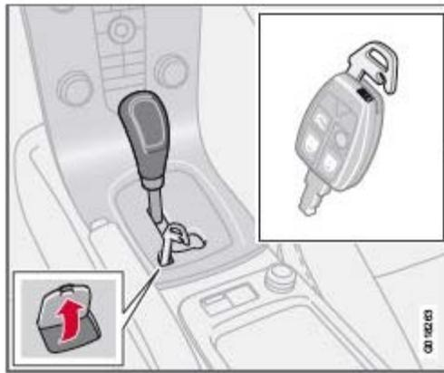
Shiftlock prevents the gear selector from being moved out of Park unless the ignition key is in position II and the brake pedal is depressed.
