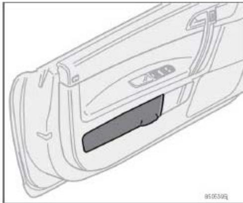
Open the compartment by lifting the front lower section of the lid.
