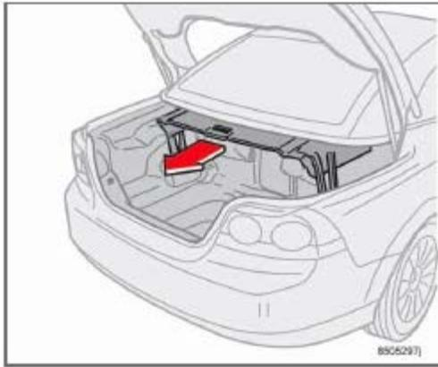
The purpose of the trunk divider is to indicate the amount of cargo that can be stowed in the trunk without affecting movement of the power retractable hard top.
