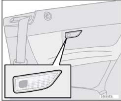
The rear reading lights can be switched on or off by pressing the respective buttons.
