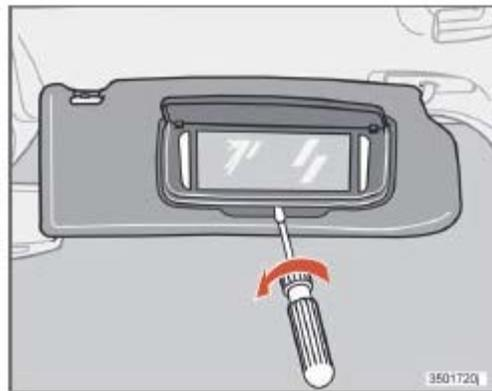
1. Insert a screwdriver under the center of the lower edge of the mirror, turn it, and carefully pry up the lugs at the edge.
