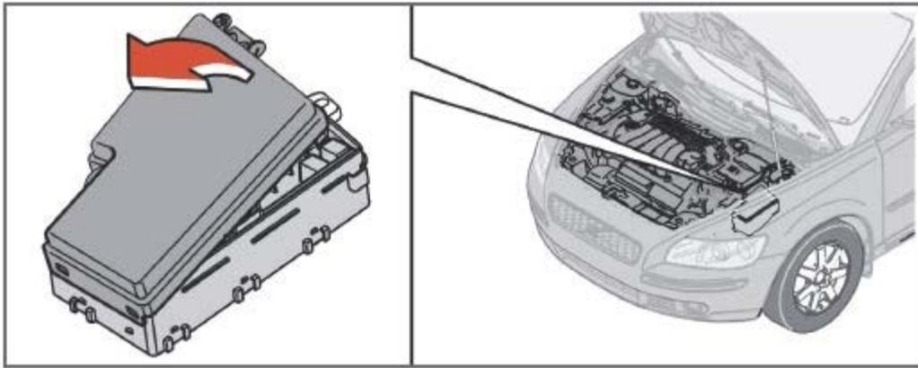
The fuse box in the engine compartment has positions for 36 fuses.
