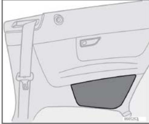
To open, press on the top center of the panel. Both the forward and rearward catches should release and the panel should spring open. If one side does not open, press again directly over that catch.
