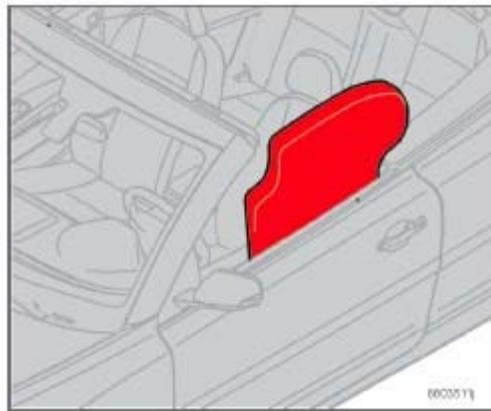
The DMIC is a supplement to the structural side impact protection. These inflatable curtains are concealed in the upper section of the driver and passenger doors.
