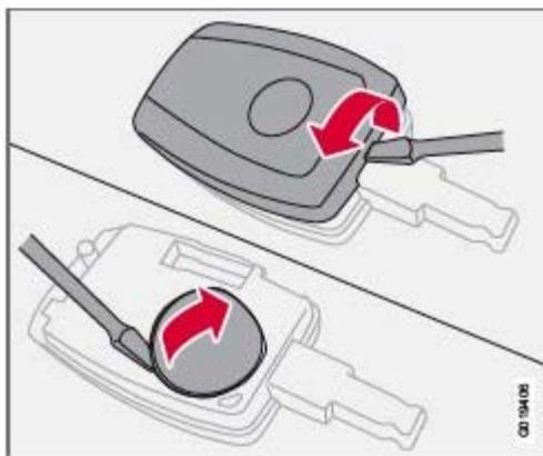
When the battery begins to lose its charge, the Information symbol in the instrument panel (see [page 49](#)) lights up and REMOTE BATTERY LOW VOLTAGE is shown in the information display.
