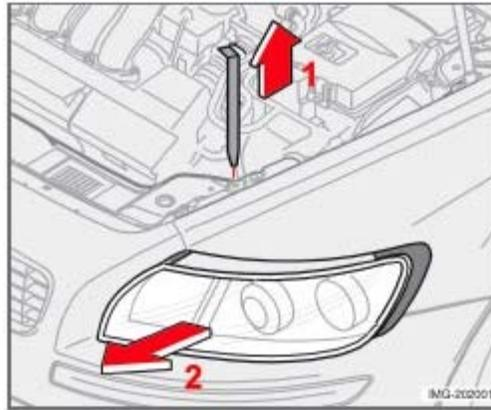
The entire headlight housing must be lifted out when replacing the high/low beam, parking light, turn signal, and side marker bulbs.
