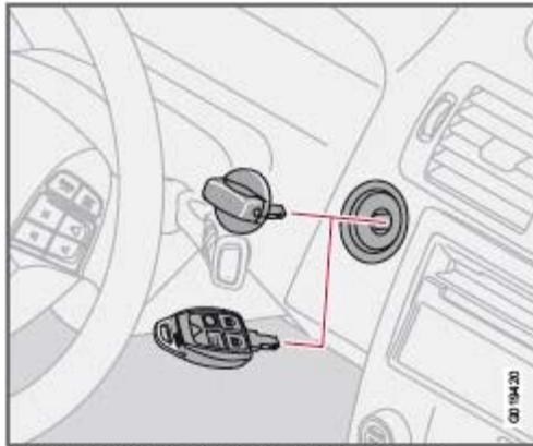
Removing the keyless drive start control
