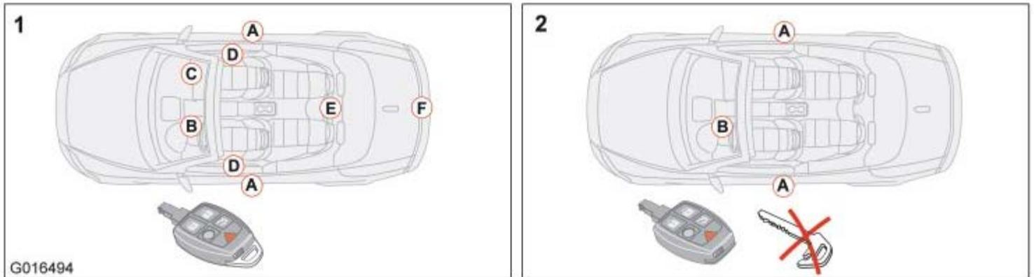
1. Locking/unlocking points for the remote control, valet locking deactivated
