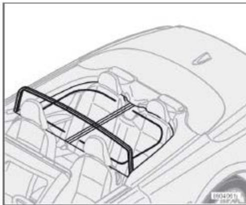
Wind blocker (retailer installed accessory)
