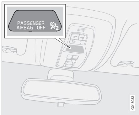
Occupant Weight Sensor (OWS) indicator light
