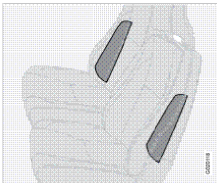
Location of the side impact (SIPS) airbag
