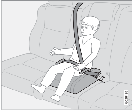
Position the child correctly on the booster cushion and positioning the seat belt
