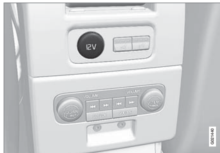
12-volt socket in the rear center console
