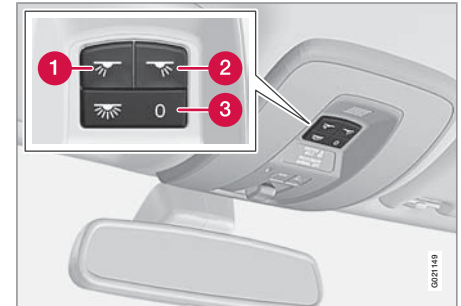
Light switches, front roof lighting
