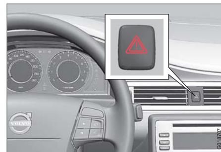
Location of the hazard warning flasher button
