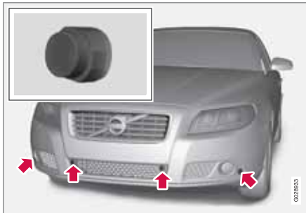
Location of the front sensors.
