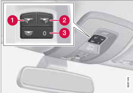
Light switches, front roof lighting
