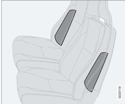
Location of the side impact (SIPS) airbag
