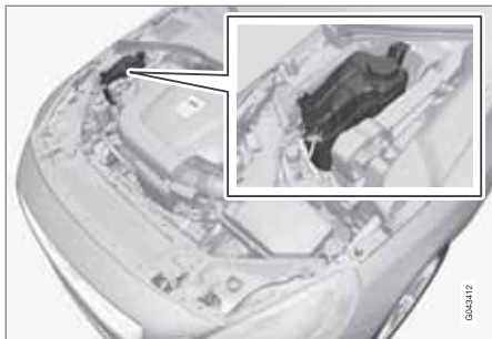
Location of the coolant reservoir
