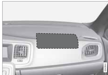
Location of the passenger's side front airbag
