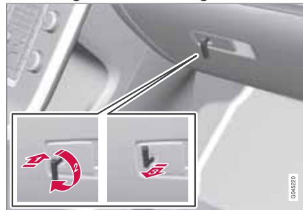
Locking/unlocking points with valet locking activated
