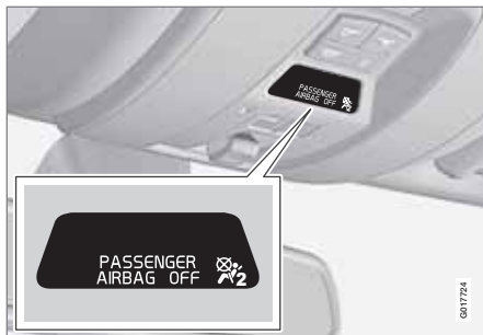
Occupant Weight Sensor (OWS) indicator light
