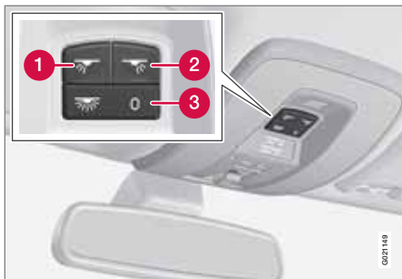
Light switches, front roof lighting
