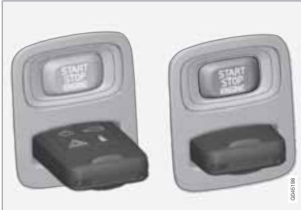
Ignition switch with remote key inserted ( see page 82 for more information on ignition modes)
