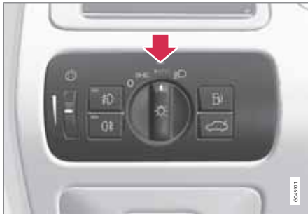
Light switch in the AUTO position
