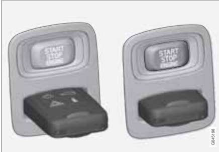
Ignition slot with remote key inserted ( see page 82 for more information on ignition modes)
