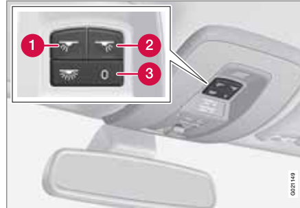
Light switches, front roof lighting
