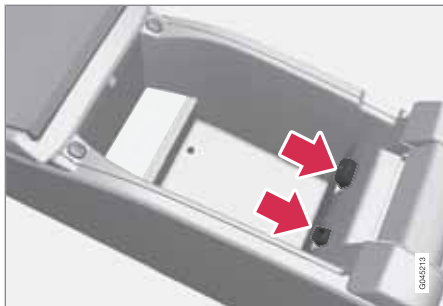
Sockets for auxiliary devices in the storage compartment between the front seats
