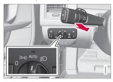
**Models with an analog instrument panel** When AHB is activated, the C symbol will illuminate in the instrument panel. The high beam indicator ( C) in the instrument panel will also illuminate when the high beams are on.
