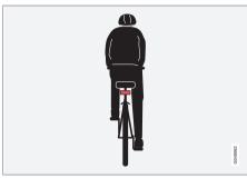
Optimal example of what the system considers to be a cyclist: clear body/bike contours, straight from behind and directly in front of the vehicle
