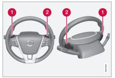
Steering-wheel mounted gear shift paddles
