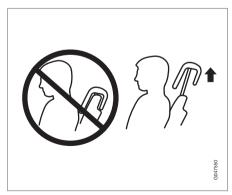
The center head restraint should be adjusted according to the passenger's height. The restraint should be carefully adjusted to support the occupant's head.
