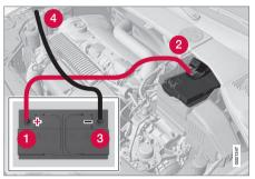
Connecting the jumper cables
