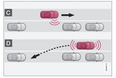
When the vehicle is backing up, PAP will steer it into the parking space.
