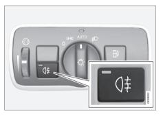
The rear fog lights will only function in combination with the high/low beam headlights.
