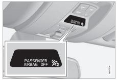
Occupant Weight Sensor (OWS) indicator light
