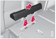
The two-sections of the net are attached to the rear side of the rear seat backrest. The cassettes have different widths, and the widest section should be mounted on the right side (seen from the rear of the vehicle).
