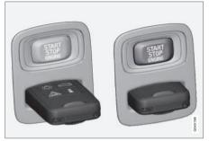
Ignition slot with remote key inserted (see Ignition modes (p. 77) for more information on ignition modes)
