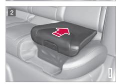
Pull the handle (1) forward and upward (2) to release the booster cushion.
