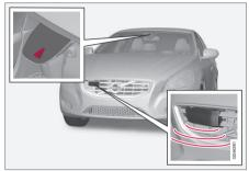
Camera and radar sensor<sup>6</sup>.
