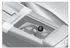
12-volt socket in the front tunnel console
