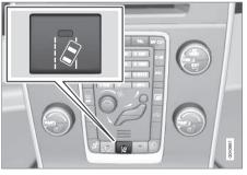
LKA can be switched on or off by pressing the button on the center console. A light in
