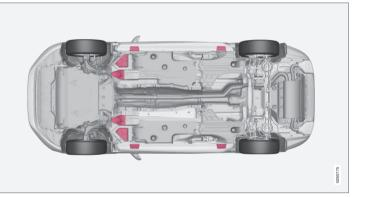
If a garage jack is used to lift the vehicle, it should be placed:
