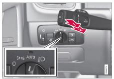
Headlight switch and steering wheel lever
