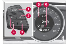
Steering wheel-mounted controls and display
