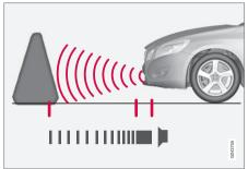
The distance monitored in front of the vehicle is approximately 2.5 ft (0.8 m). The audible signal comes from the audio system's front speakers.
