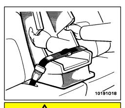
Make sure the seat belt is securely locked. Also make sure the child restraint system is secure by pushing and pulling it in different directions.
