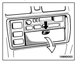
To open the miscellany box, press on the knob and pull out the box lid.
