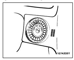
For easy access to the ignition switch, the ignition switch light comes on when any of the side doors are opened.
