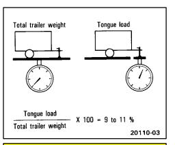
• The trailer cargo load should be distributed so that the tongue load is 9 to 11 % of the total trailer weight, not exceeding the maximum of 90 kg (200 lb.). Never load the trailer with more weight in the back than in the front. About 60 % of the trailer load should be in the front half of the trailer and the remaining 40 % in the rear.
