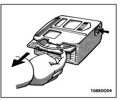
3. While pressing the lock release button on the magazine, draw out a tray.
