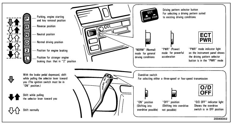
When the cruise control is being used, even if you downshift the transmission by turning off the overdrive switch, engine braking will not be applied because the cruise control is not cancelled. For ways to decrease the vehicle speed, see "Cruise control" in this chapter.
