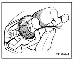
The SRS (Supplemental Restraint System) airbags are designed to provide further protection to occupants in the following seats when added to the primary protection provided by the seat belts.
