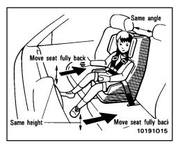
If your driving position is not satisfactory, or the child restraint system interferes with your driving, install it at another position.
