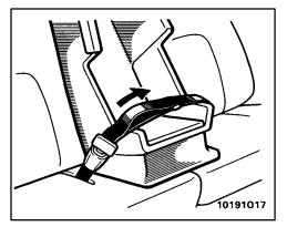
2. To hold the child restraint system securely, tighten the belt by pulling its free end while firmly pushing down the child restraint system.
