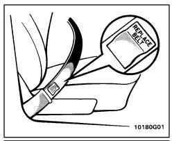
• Front passenger's seat only (except the center position of bench front seat). Replace the belt if the warning label under the sleeve can be seen. The warning label, "RE-PLACE BELT", will appear if the belt receives a severe impact or other force.
