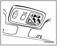
To turn on the front personal lights, push the switch. To turn the lights off, push the switch once again.
