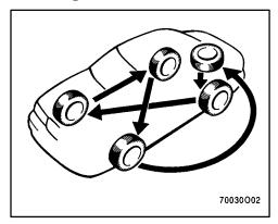
To equalize tire wear and help extend tire life, Toyota recommends that you rotate your tires every 12000 km (7500 miles). However, the most appropriate timing for tire rotation may vary according to your driving habits and road surface conditions.
