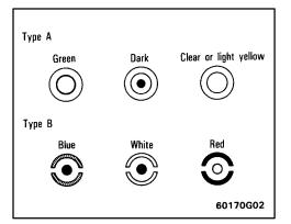
CHECKING BY THE HYDROMETER Check the battery condition by the hydrometer color.
