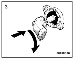
3. Install a new bulb and the connector into the mounting hole.
