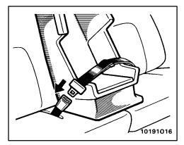
1. Fasten the lap and shoulder belt over the child restraint system following the instructions provided by its manufacturer.
