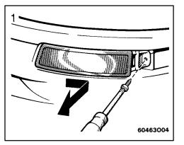
Remove the front side marker unit. Use a Phillips-head screwdriver.
