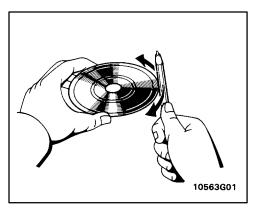
A new disc may have rough edges on its inner and outer perimeter. Remove the rough edges by pressing the side of a ball-point pen or pencil against the inner and outer perimeter of the disc as shown.
