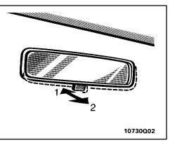
To reduce glare from the headlights of the vehicle behind you during night driving, operate the lever on the lower edge of the mirror.
