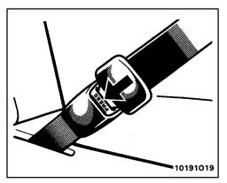
3. To remove the child restraint system, press the buckle-release button and unhook the top strap.
