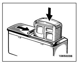
5. Insert the magazine into the automatic changer as shown above. Then close the cover.
