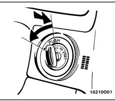
"START"—Starter motor on. The key will return to the "ON" position when released.
