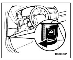
To open the hood, do the following. 1. Pull the hood lock release lever. The hood will spring up slightly.
