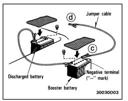
c. Connect the clamp of the negative (black) cable to the negative (-) terminal on the booster battery.
