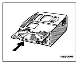
4. Place a disc on the tray with its label face up, and insert the tray into the slot.
