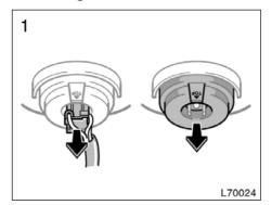
1. Open the hood. Unplug the connector. Remove the rubber cover.
