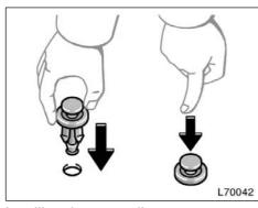
Installing the cover clips
