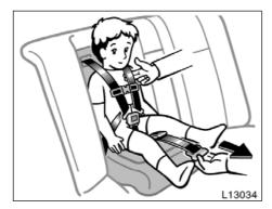
9. Pull the seat belt adjustment strap (gray tab) firmly until the shoulder belts are snugly adjusted around the child's shoulders.
