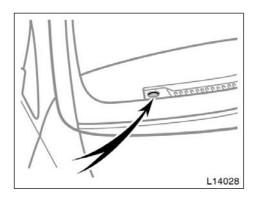
The daytime running light control sensor is on the top of the passenger's side instrument panel.
