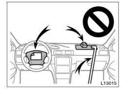
• Do not put objects or your pets on or in front of the dashboard or steering wheel pad that houses the airbag system. They might restrict inflation or cause death or serious injury as they are projected rearward by the force of deploying airbags. Likewise, the driver and front passenger should not hold things in their arms or on their knees.
