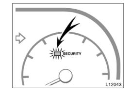
The system is automatically set when the key is removed from the ignition switch. The indicator light will start flashing every 1 second to show the system is set.
