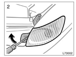
Use a flat-bladed screw driver. To protect the surface, place several sheets of paper over the surface.
