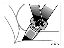
To remove the infant seat, press the buckle-release button and allow the belt to retract completely. The belt will move freely again and be ready to work for an adult or older child passenger.
