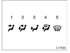
Turning the Air Flow Selector to windshield position turns on the defroster to clear the front view more quickly.
