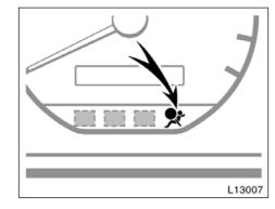
This SRS side airbag system has a service reminder indicator to inform the driver of operating problems. If either of the following conditions occurs, this indicates a malfunction of the airbags. Contact your Toyota dealer as soon as possible to service the vehicle.
