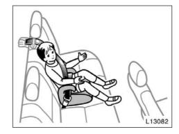
(C) BOOSTER SEAT INSTALLATION A booster seat is used in forward-facing position only.
