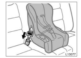
1. Run the lap and shoulder belt through or around the convertible seat following the instructions provided by its manufacturer and insert the tab into the buckle taking care not to twist the belt. Keep the lap portion of the belt tight.
