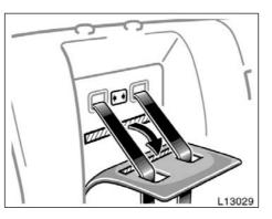
5. Pull down the seatback part of the removable pad. Make sure the child's shoulders are at or below the maximum shoulder height indicator label.
