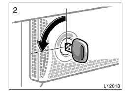
2. After closing the trunk lid, insert the master key and turn it counterclockwise to deactivate the lock release lever.
