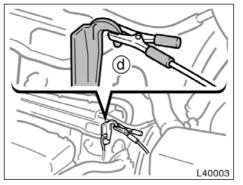
Connecting point for 5S-FE engine
