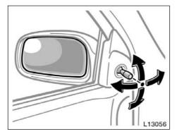
To adjust the rear view mirror, simply operate the control lever.
