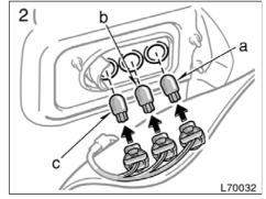
a: Rear side marker light b: Rear turn signal light c: Stop and tail light
