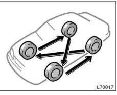
To equalize the wear and help extend tire life, Toyota recommends that you rotate your tires approximately every 12000 km (7500 miles). However, the most appropriate timing for tire rotation may vary according to your driving habits and road surface conditions.
