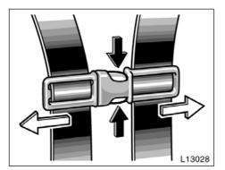
4. Compress the shoulder belt clip to separate the right and left shoulder belts.
