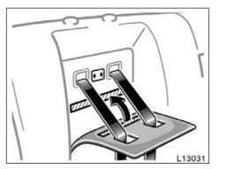
6. Press the removable pad against the fastener tapes and install the pad to the seatback. Make sure the belts go through the slots in the pad.
