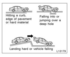
The SRS airbags may deploy if a serious impact occurs to the underside of your vehicle. Some examples are shown in the illustration.
