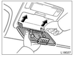
The miscellaneous box and garage door opener box (stored in the glove box) are interchangeable.
