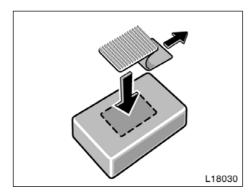
Remove the paper strip covering the adhesive on back side of loop and adhere loop to back side of the transmitter near center.
