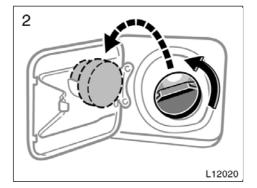
2. To remove the fuel tank cap, turn the cap slowly counterclockwise, then pause slightly before removing it. After removing the cap, hang it on the cap hanger.
