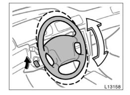
To change the steering wheel angle, hold the steering wheel, pull up the lock release lever, tilt the steering wheel to the desired angle and release the lever.
