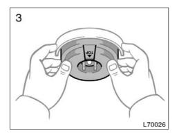
3. Install the rubber cover with the "TOP" mark upward, and snuggle on the boss. Insert the connector. Then install the plastic cover.
