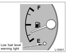
The gauge works when the ignition switch is on and indicates the approximate quantity of fuel remaining in the tank.
