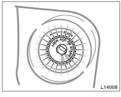
For easy access to the ignition switch, the ignition switch light comes on when any of the doors are opened.
