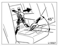
3. While pulling the seat belt release strap (black), pull both shoulder belts together.
