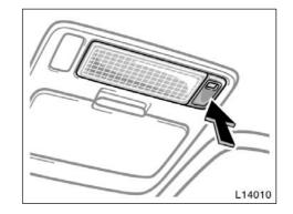
To turn on the personal light, push the switch. To turn it off, push the switch once again.
