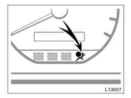
This indicator comes on when the ignition key is turned to the "ACC" or "ON" position. It goes off after about 6 seconds. This means the SRS airbags are operating properly.
