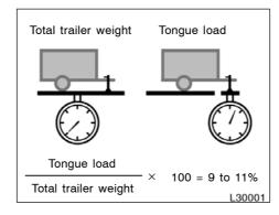
• The trailer cargo load should be distributed so that the tongue load is 9 to 11% of the total trailer weight, not exceeding the maximum of 90 kg (200 lb.). Never load the trailer with more weight in the back than in the front. About 60% of the trailer load should be in the front half of the trailer and the remaining 40% in the rear.
