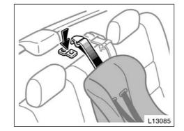
If your child restraint system requires the use of a top strap, latch the hook onto the anchor bracket and tighten the top strap.
