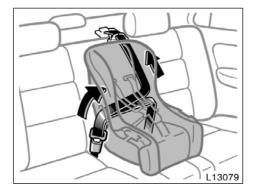
3. While pressing the convertible seat firmly against the seat cushion and seatback, let the shoulder belt retract as far as it will go to hold the convertible seat securely.
