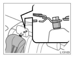
To comply with Canadian Motor Vehicle Safety Standards, this model sold in Canada is provided with a bracket set in the glovebox, designed for use with any of the 3 anchor locations shown in the illustration.
