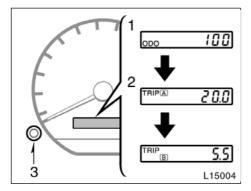
This meter displays the odometer and two trip meters.
