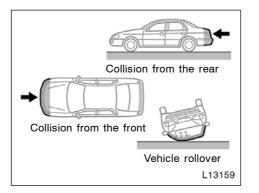
The SRS side airbags are not designed to inflate if the vehicle is subjected to a front or rear impact, if it rolls over, or if it is involved in a low-speed side collision.
