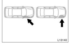
The SRS side airbags may not inflate if the vehicle is subjected to a collision from the side at an angle, or a collision to the side of the vehicle body other than the passenger compartment shown in the illustration, which impact is not severe enough for the passenger compartment.
