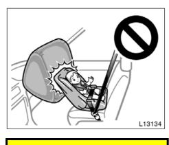
• Never put a rear-facing child restraint system on the front seat because the force of the rapid inflation of the passenger airbag can cause death or serious injury to the child.
