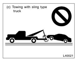
(c) Towing with sling type truck
