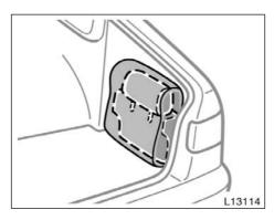
2. Insert the head restraint and upper pad into the storage bag. Then place the storage bag into the trunk by attaching with Velcro.
