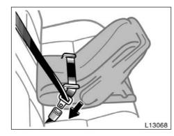
1. Run the lap and shoulder belt through or around the infant seat following the instructions provided by its manufacturer and insert the tab into the buckle taking care not to twist the belt. Keep the lap portion of the belt tight.
