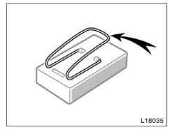
Please note if transmitter has wire clip for sun visor, this clip must be removed prior to adhesion of the Velcro.
