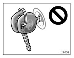
When starting the engine, do not use the key with other transponder keys around (including keys of other vehicles) and do not press other key plates against the key grip. Otherwise the engine may not start, or may stop soon after it starts. If this happens, remove the key once and then insert it again after taking off other transporter keys (including keys of other vehicles) from the ring or while gripping or covering them with your hand to start the engine.
