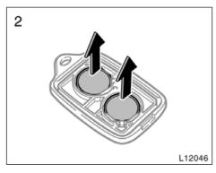
2. Remove the discharged transmitter batteries.
