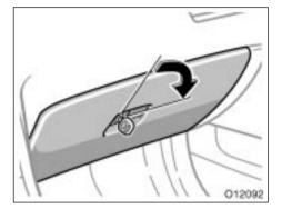
This system helps protect things locked in the trunk by safeguarding the lock release switch from unwanted access.
