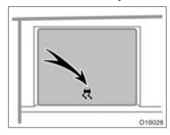
The vehicle skid control system helps provide comprehensive control of the systems such as an anti-lock brake system, brake assist system, traction control, engine control, etc. This system automatically controls the output of the brakes or engine to help prevent the vehicle from skidding when cornering on a slippery road surface or abrupt steering wheel operation occurs. If the vehicles is going to skid during driving, the slip indicator light flashes and an alarm sounds intermittently.
