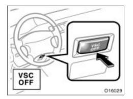
You can turn off the traction control system by pushing the "VSC OFF" switch. The "VSC OFF" indicator light will come on. Pushing the "VSC OFF" switch a second time turns on the traction control system again and the "VSC OFF" indicator light will go off. At this time, the vehicle skid control also turns off and on simultaneously.
