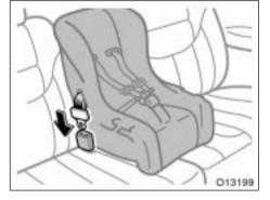
1. Run the center lap belt through or around the convertible seat following the instructions provided by its manufacturer and insert the tab into the buckle taking care not to twist the belt. Keep the lap portion of the belt tight.
