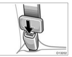
3. To remove the convertible seat, press the buckle-release button and allow the belt to retract completely. The belt will move freely again and be ready to work for an adult or older child passenger.
