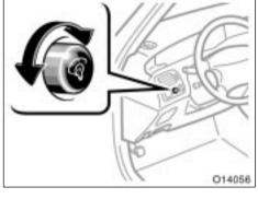
To adjust the brightness of the instrument panel lights, turn the knob. Front fog lights
