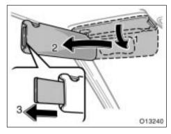
To block out glare, move the sun visor. To block out glare from the front—Swing down the main sun visor
