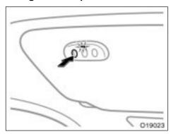
Garage door openers manufactured under the license from HomeLink<sup>®</sup> and can be programmed to operate garage doors, estate gates, security lighting, etc.
