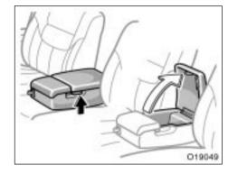
To use the box, pull up the lock release lever and open the lid.
