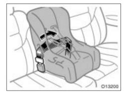
2. While pressing the convertible seat firmly against the seat cushion and seatback, tighten the lap belt by pulling its free end to hold the convertible seat securely.
