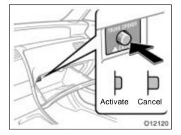
If you do not want to activate the trunk lid opener system, turn off the trunk opener cancel switch in the glove box. To turn it on, push in the trunk opener cancel switch.
