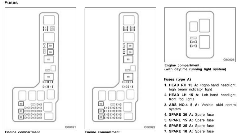
Engine compartment (without daytime running light system) Engine compartment (with daytime running light system)
