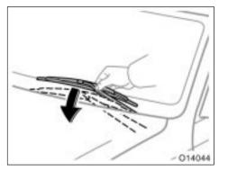
To replace the windshield wipers to the retracted position, push the connection of the wiper arm and wiper blade downward.
