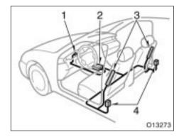
The SRS side airbag system may not activate if the vehicle is subjected to a collision from the side at certain angles, or a collision to the side of the vehicle body other than the passenger compartment as shown in the illustration.
