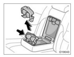
To maximize the storage room, remove the cup holder by pushing the side facing at its upright position.
