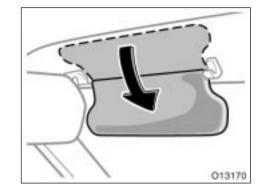
To block the glare from the front when the main sun visor is swung to the side, swing down the second sun visor
