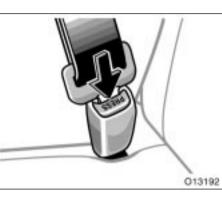
Push and pull the child restraint system in different directions to be sure it is secure. Follow all the installation instructions provided by its manufacturer. 4. To remove the convertible seat, press the buckle-release button and allow the belt to retract completely. The belt will move freely again and be ready to work for an adult or older child passenger.
