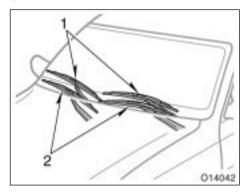
The wiper blades retract under the hood when the wipers are turned off. If retraction is obstructed by snow, etc., at the bottom of the windshield, the wipers should be shifted from the retracted position (position 2) to the rest position (position 1) above the hood level. When the snow season is over, manually return the wipers to the retracted position following the procedure given below.
