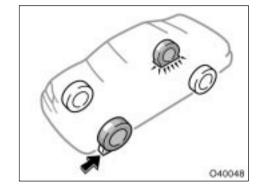
2. Block the wheel diagonally opposite the flat tire to keep the vehicle from rolling when it is jacked up.
