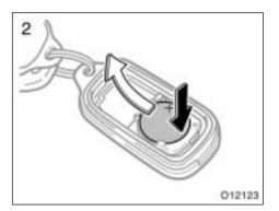
2. Push the edge of the discharged transmitter battery and lift it out as shown in the above illustration.
