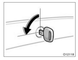
This system deactivates the lock release switch so that things locked in the trunk can be protected.
