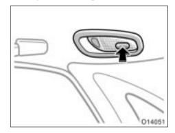
To turn on the rear personal light, push the switch. To turn the light off, push the switch once again.
