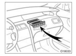
Automatic air conditioning system only—This air conditioning system has a high efficient air refiner filter which helps eliminate dust and pollen, thereby increasing your driving confort.
