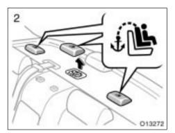
2. Remove the anchor bracket cover with the symbol mark shown in the illustration.
