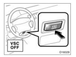
You can turn off the vehicle skid control system by pushing the "VSC OFF" switch. The "VSC OFF" indicator light will come on. Pushing the "VSC OFF" switch a second time turns the system again and the "VSC OFF" indicator light will go off. At this time, the traction control also turns off and on simultaneously.
