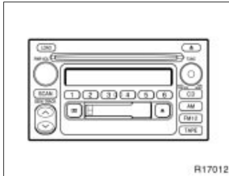
Type 4: AM-FM ETR radio/cassette player/ compact disc auto changer controller/ compact disc auto changer
