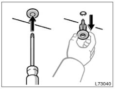
Removing the cover clips (Type A)
