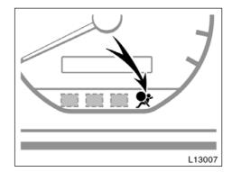
This SRS front airbag system has a service reminder indicator to inform the driver of operating problems. If either of the following conditions occurs, this indicates a malfunction of the airbags. Contact your Toyota dealer as soon as possible to service the vehicle.
