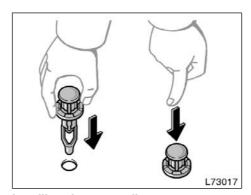
Installing the cover clips
