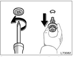
Removing the cover clips (Type B)
