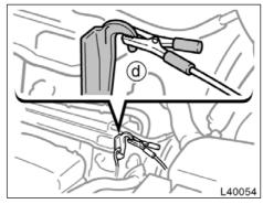
Connecting point for 5S-FE engine
