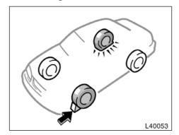
Block the wheel diagonally opposite the flat tire to keep the vehicle from rolling when it is jacked up.
