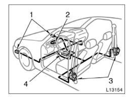
The front seat belt pretensioner system mainly consists of the following components and their locations are shown in the illustration.
