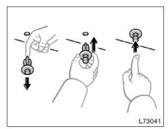
Installing the cover clips (Type A)
