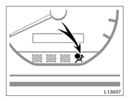
This indicator comes on when the ignition key is turned to the "ACC" or "ON" position. It goes off after about 6 seconds. This means the front seat belt pretensioners are operating properly.
