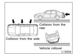
The SRS front airbags are not designed to inflate if the vehicle is involved in a side or rear collision, if it rolls over, or if it is involved in a low-speed frontal collision.
