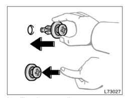
Installing the cover clips
