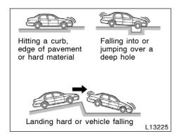
The front SRS airbags may deploy if a serious impact occurs to the underside of your vehicle. Some examples are shown in the illustration.
