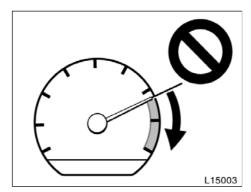
The tachometer indicates engine speed in thousands of rpm2(revolutions per minute). Use it while driving to select correct shift points and to prevent engine lugging and over-revving.
