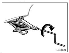
After making sure that no one is in the vehicle, raise it high enough so that the spare tire can be installed.
