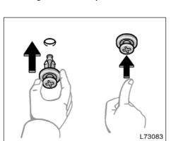
Installing the cover clips
