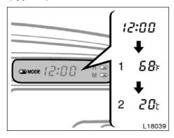
The outside temperature gauge indicates the outside air temperature.
