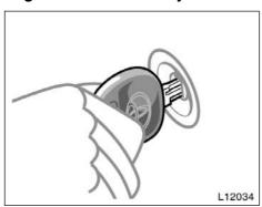
The engine immobiliser system is a theft prevention system. When you insert the key in the ignition switch, the transporter chip in the key's head transmits an electronic code to the vehicle. The engine will start, only when the electronic code in the chip corresponds to the registered ID code for the vehicle.
