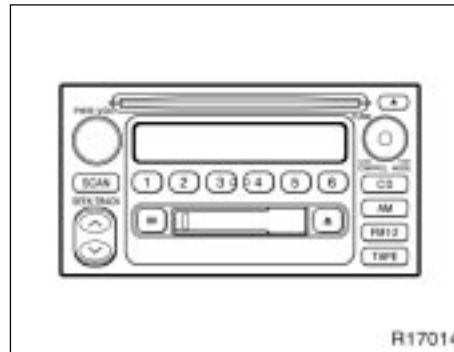
Type 3: AM-FM ETR radio/cassette player/compact disc player (with compact disc auto changer controller)
