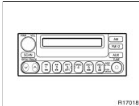
Type 1: AM-FM ETR radio (with cassette and compact disc auto changer controllers)
