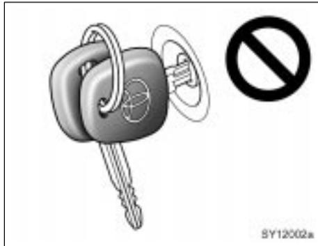
◆ **When starting the engine, do not use the key with other transponder keys around (including keys of other vehicles) and do not press other key plates against the key grip. Otherwise the engine may not start, or may stop soon after it starts. If this happens, remove the key once and then insert it again after taking off other transponder keys (including keys of other vehicles) from the ring or while gripping or covering them with your hand to start the engine.**
