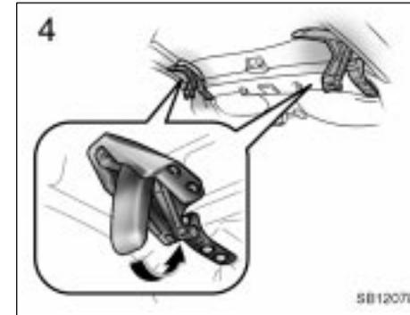
4. Keep pressing the soft top against the frame of the front window glass and fix the soft top by pushing up the right and the left lock levers until a click is heard.
