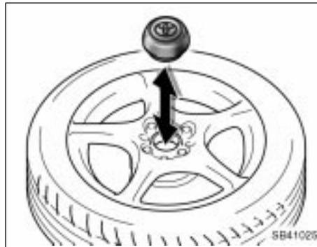
Remove the wheel ornament from the flat tire before restoring the flat tire.
