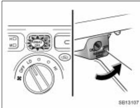
When you put a forward-facing child restraint system which belongs to passenger risk group on the passenger seat, turn the passenger airbag manual on-off switch counterclockwise to the "OFF" position. (For details, see "SRS driver and passenger airbags" on page 36 in this section.)
