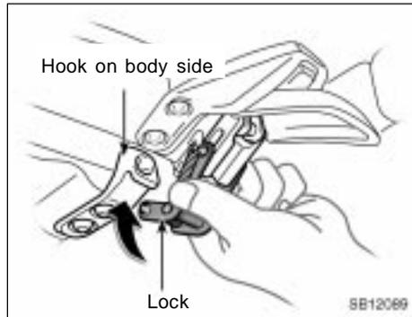
**If the lock is not hung easily, give your hand to the lock for helping to hang it on the hook on the body side.**
