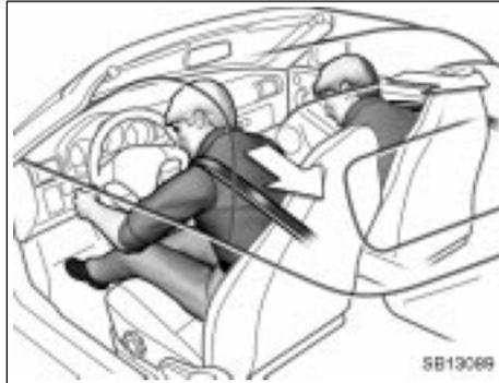
The driver and passenger's seat belt pretensioners are designed to be activated in response to a severe frontal impact.
