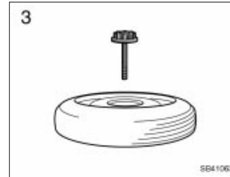
3. Loosen the bolt and remove it.
