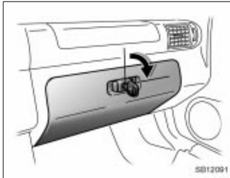
If you do not want to activate the trunk lid lock release lever, insert the master key to the glove box, and turn it clockwise.
