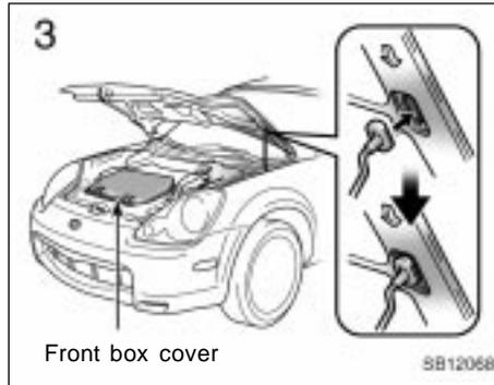
3. Hold the trunk lid open by inserting the support rod into the slot.
