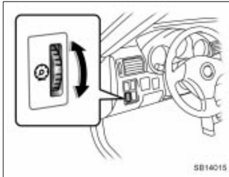
To adjust the brightness of the instrument panel lights, turn the switch.
