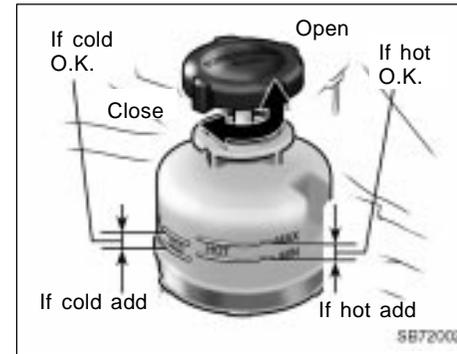
Check the fluid level through the reservoir. If necessary, add Toyota P.S fluid EH or equivalent.
