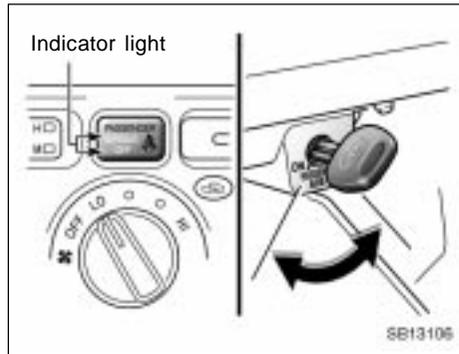
This on-off switch is designed to disable the passenger airbag in order to allow usage, if necessary, of a member of a passenger risk group identified in TABLE 1 (on page 38) is occupying the passenger seating position (For details, see “SRS driver and passenger airbags” on page 36 in this section.)
