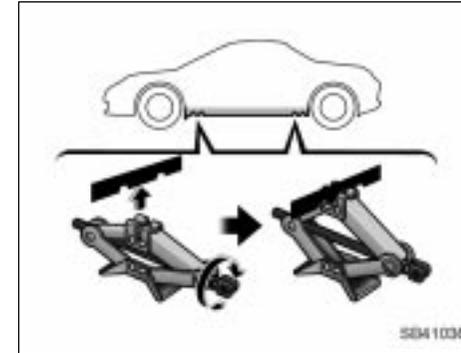
**4. Position the jack at the correct jacking point as shown.**
