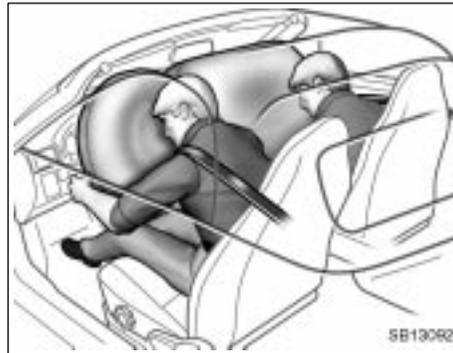
**The SRS (Supplemental Restraint System) airbags are designed to provide further protection for the driver and passenger in addition to the primary safety protection provided by the seat belts.**
