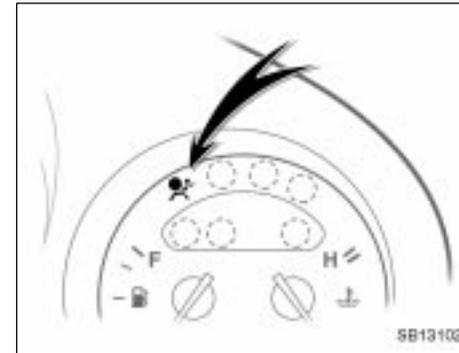
This seat belt pretensioner system has a service reminder indicator to inform the driver of operating problems. If any of the following conditions occurs, this indicates a malfunction of the airbags or pretensioners. Contact your Toyota dealer as soon as possible to service the vehicle.
