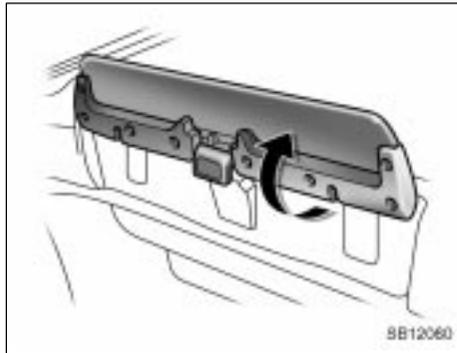
The air deflector will reduce the wind from the rear of the vehicle when the vehicle is running with the soft top lowered. Pull up to use.
