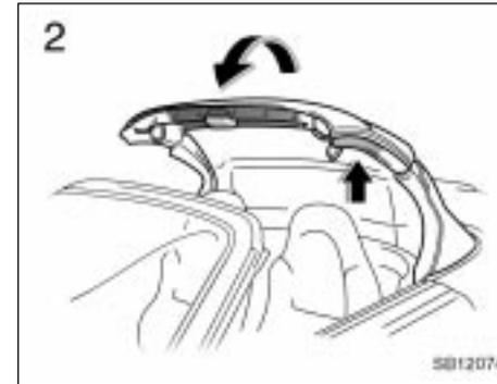
2. Stand outside of the vehicle and pull the soft top out slowly holding the part shown in dark color in the illustration. Then move the soft top toward the upper part of the frame of the front window glass.
