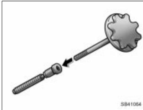
When you store the replaced flat ground tire in the place where the compact spare tire was loaded, install the spare wheel extension to the spare wheel clamp.
