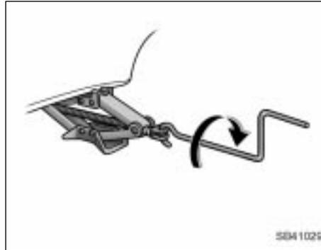
**5. After making sure that no one is in the vehicle, raise it high enough so that the compact spare tire can be installed.**
