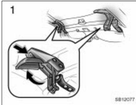
1. Lower both side windows and sun visors. Then pull down the lock levers on both sides of the vehicle fully while pushing down the button.
