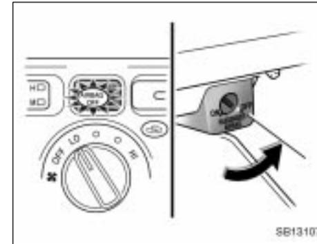
When you put a forward-facing or a rear-facing child restraint system which belongs to a passenger risk group on the passenger seat, turn the passenger airbag manual on-off switch counter-clockwise to the "OFF" position. (For details, see "SRS driver and passenger airbags" on page 36 in this section.)
