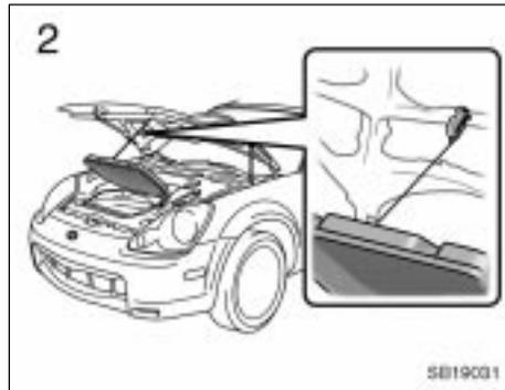
2. Fix the cover by hitching the inside clip on the hood.
