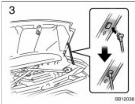
**3. Hold the engine hood open by inserting the support rod into the slot.**
