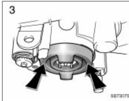
**3. Install the rubber cover as shown and snuggle on the boss. Plug in the connector.**
