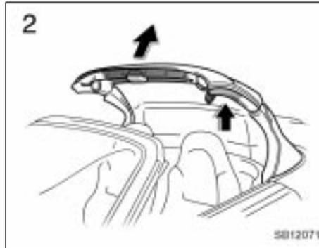
2. Stand outside of the vehicle and pull the soft top up holding the part shown in dark color in the illustration.
