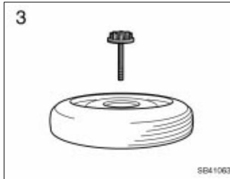
3. Loosen the bolt and remove it.
