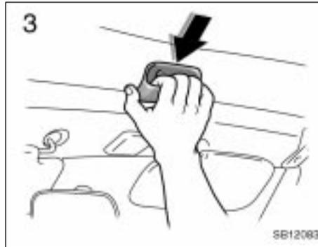
3. Be seated in the seat and hold the handle on the center of the front soft top frame. Then press the soft top softly against the frame of the front window glass.
