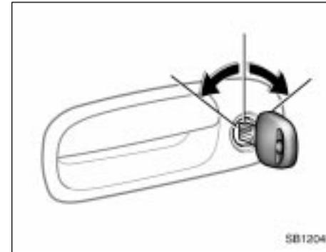
**LOCKING AND UNLOCKING WITH KEY**
