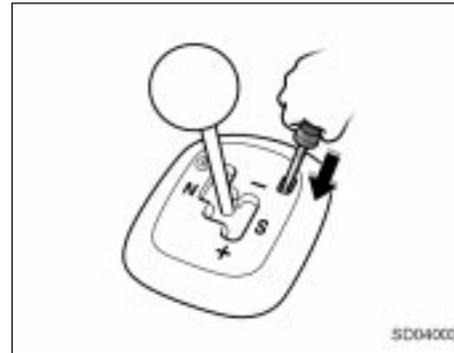
3. To push the link, insert a key or screwdriver to the hole. The lever can be operated while the link is being pushed.
