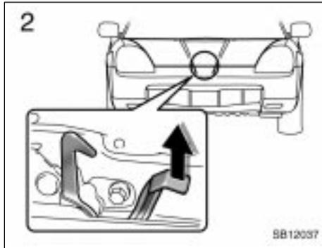
2. In front of the vehicle, pull up the auxiliary catch lever and lift the trunk lid.
