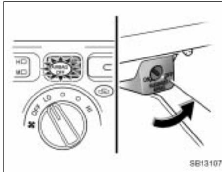
When you put a rear-facing child restraint system which belongs to a passenger risk group on the passenger seat, turn the passenger airbag manual on-off switch counterclockwise to the "OFF" position. (For details, see "SRS driver and passenger airbags" on page 36 in this section.)
