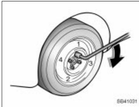
**8. Lower the vehicle completely and tighten the wheel nuts.**
