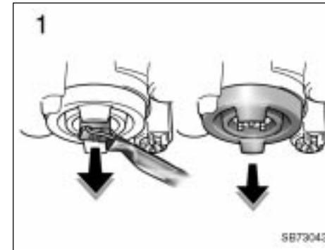
**1. Unplug the connector. Remove the rubber cover.**
