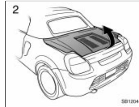
2. In rear of the vehicle, lift the engine hood.
