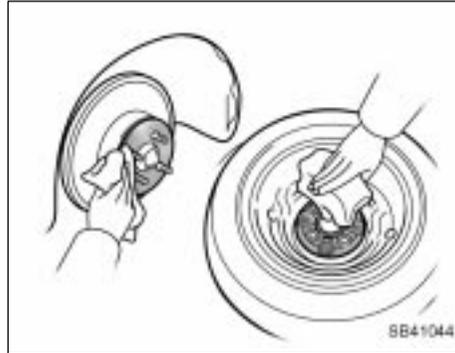
Before putting wheels on, remove any corrosion on the mounting surfaces with a wire brush or such. Installation of wheels without good metal-to-metal contact at the mounting surface can cause wheel nuts to loosen and eventually cause a wheel to come off while driving. Therefore after the first 1600 km (1000 miles), check to see that the wheel nuts are tight.
