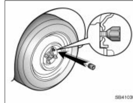
**7. Reinstall all the wheel nuts with finger tight.**
