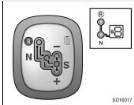
The sequential manual transmission has a shift lock system. This system locks the selector lever to keep the transmission gear and the selector lever position in the same position when the ignition switch is turned to the “ACC” or “LOCK” position. However, if the selector lever is locked in the “S” position, the lever can be moved to the “+” or “-” direction, but the gear will not be actually shifted.
