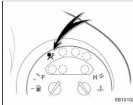
This SRS airbag system has a service reminder indicator to inform the driver of operational problems. If either of the following conditions occurs, this indicates a malfunction of the airbags. Contact your Toyota dealer as soon as possible to service the vehicle.
