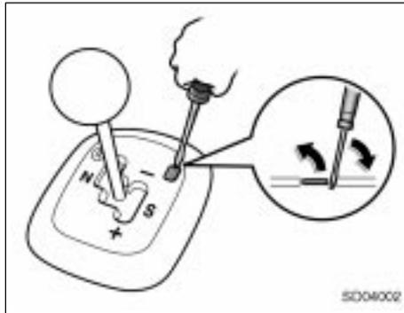
In case the selector lever lock is not released and the selector lever cannot be moved even though the ignition switch is turned to the "ON" position, follow the procedures below:
