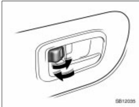
**LOCKING AND UNLOCKING WITH INSIDE LOCK KNOB**
