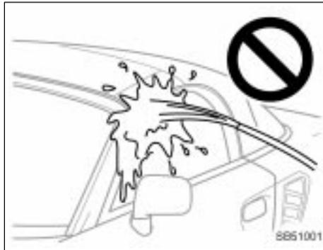
Spray water on the side windows or top seals from above, at a 45° angle to the ground.
