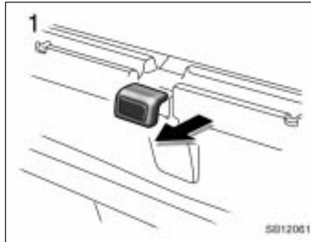
1. Lower both side windows and sun visors. Then pull down the lock release lever towards the front of the vehicle and release the lock of the soft top.
