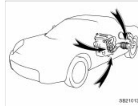
The three-way catalytic converter is an emission control device installed in the exhaust system.
