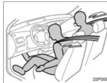
The driver and front passenger's seat belts pretensioners are designed to be activated in response to a severe frontal impact.
