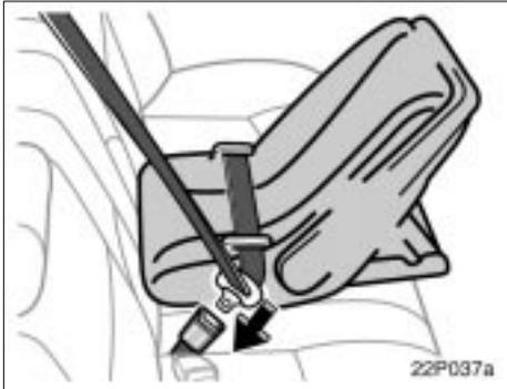
1. Run the lap and shoulder belt through or around the baby seat following the instructions provided by its manufacturer and insert the tab into the buckle taking care not to twist the belt. Keep the lap portion of the belt tight.
