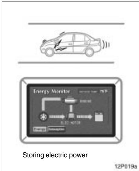
**When decreasing speed or applying the brakes,** the turning force of the wheels makes the electric motor operate as a generator and additional electricity is stored in the hybrid vehicle battery (regenerative brake).
