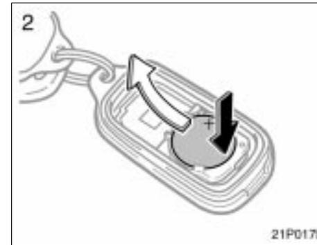
2. Remove the discharged transmitter battery.
