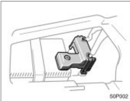
5. Remove the positive terminal cover of the auxiliary battery.
