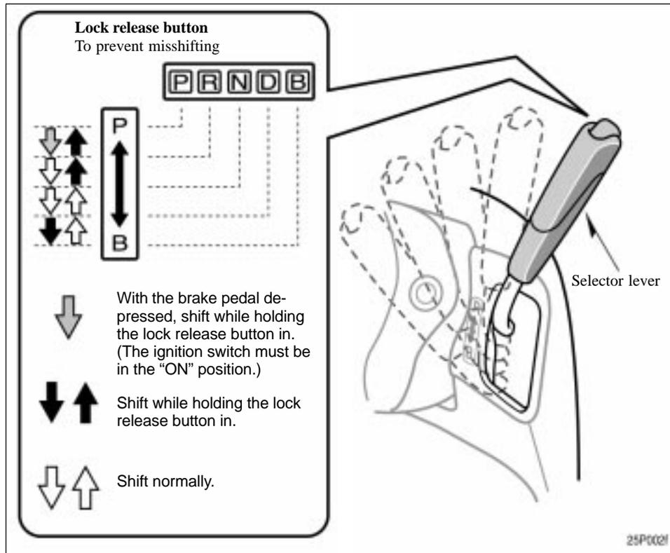
Your hybrid transaxle has a shift lock system to minimize the possibility of incorrect operation. This means you can only shift out of "P" position when the brake pedal is depressed (with the ignition switch in "ON" position and the lock release button depressed).
