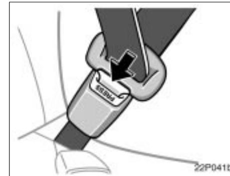
4. To remove the baby seat, press the buckle-release button and allow the belt to retract completely. The belt will move freely again and be ready to work for an adult or older child passenger.
