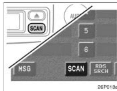
**Scan tuning:** Push the “SCAN” button or touch the “SCAN” switch briefly. “SCAN” appears on the display. The radio will find the next station up or down the band, stay there for a few seconds, and then scan again. To select a station, push the “SCAN” button or touch the “SCAN” switch a second time.
