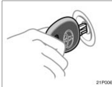
The hybrid vehicle immobiliser system is a theft prevention system. When you insert the key in the ignition switch, the transponder chip in the key's head transmits an electronic code to the vehicle. The hybrid system will start, only when the electronic code in the chip corresponds to the registered ID code for the vehicle.
