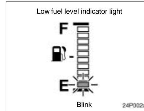
If the fuel level approaches “E” or the low fuel level indicator light blinks, fill the fuel tank as soon as possible.
