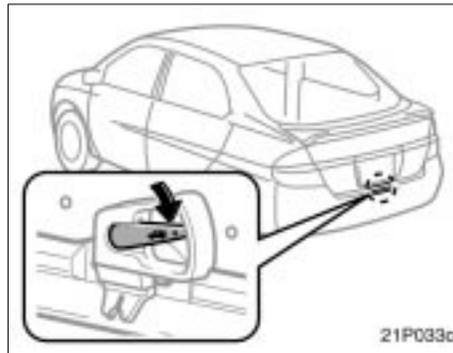
If a person is locked in the trunk, he or she can pull down the phosphorescent handle on the inside of trunk lid in case of emergency to open the trunk lid.
