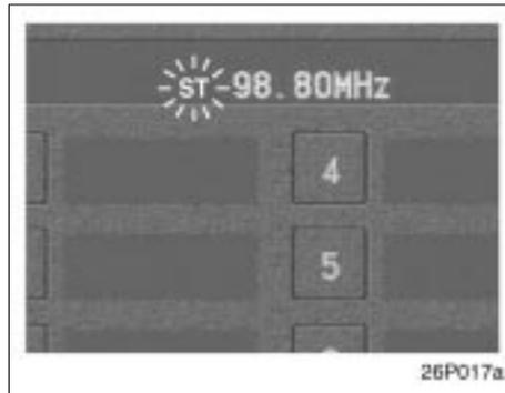
Your radio automatically changes to stereo reception when a stereo broadcast is received. “ST” appears on the display. If the signal becomes weak, the radio reduces the amount of channel separation to prevent the weak signal from creating noise. If the signal becomes extremely weak, the radio switches from stereo to mono reception. In this case, “ST” disappears from the display.
