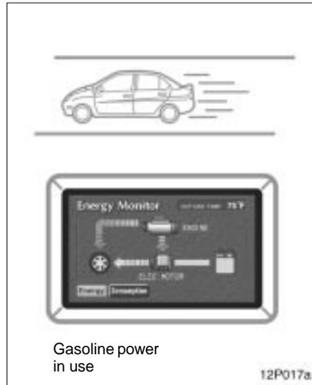
**During normal driving,** the vehicle runs mainly on gasoline power. However, the electric motor, using electric power generated by the gasoline engine, makes up for any deficiency of gasoline power.
