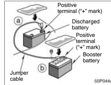
9. Connect the jumper cables in the order a, b, c, d.
