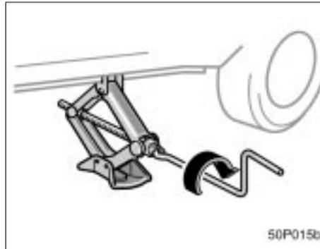
5. After making sure no one is in the vehicle, raise it high enough so that the spare tire can be installed.
