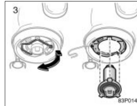
**3. Release the bulb retaining spring and remove the bulb along with the socket. Install a new bulb into the socket and return the bulb retaining spring to its original position.**
