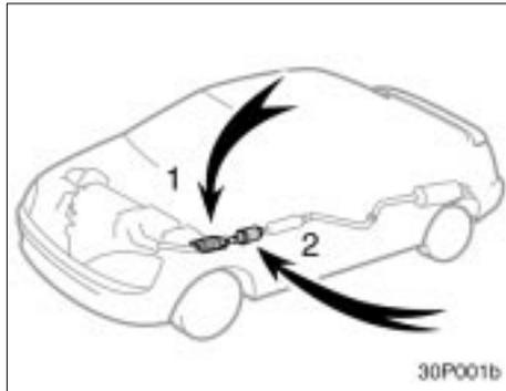
1. Three-way catalytic converter
