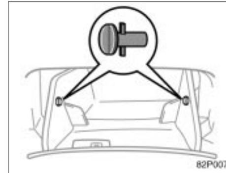
1. Open the glove box. Turn and pull out 2 pins located on both sides. Pull down the glove box.
