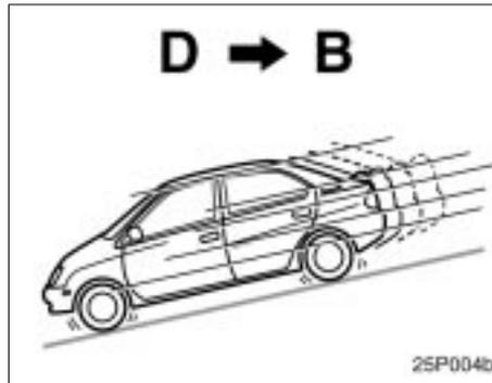
**(c) Using engine braking**
