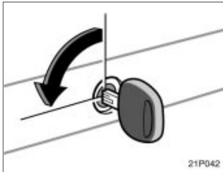
After closing the trunk lid, insert the master key and turn it counterclockwise to deactivate the lock release lever.
