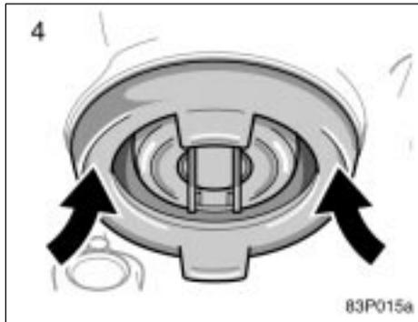
**4. Install the rubber cover as shown, and snuggle on the boss. Plug in the connector.**
