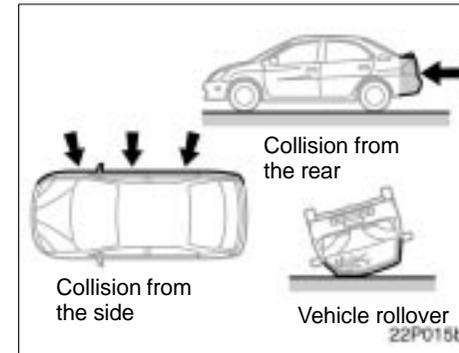
**The SRS front airbags are not designed to inflate if the vehicle is involved in a side or rear collision, if it rolls over, or if it is involved in a low-speed frontal collision.**
