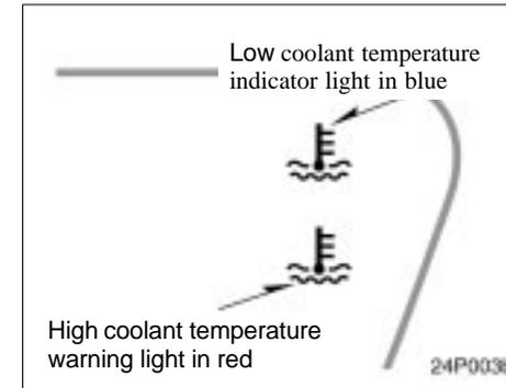
The indicator and warning lights indicate the coolant temperature when the ignition switch is on. The hybrid system operating temperature will vary with changes in weather and hybrid system load.
