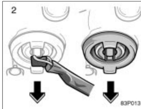
**2. Unplug the connector. Remove the rubber cover.**
