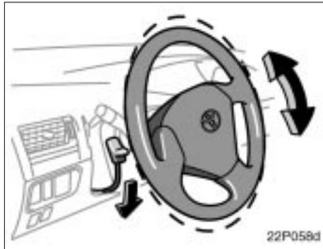
To change the steering wheel angle, hold the steering wheel, push down the lock release lever, tilt the steering wheel to the desired angle and push the lever up to lock the steering wheel in position.
