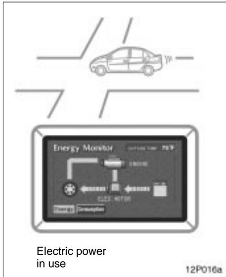
**When starting or backing up, etc., the gasoline engine efficiency worsens,** so the vehicle runs on electric power from hybrid vehicle battery.
