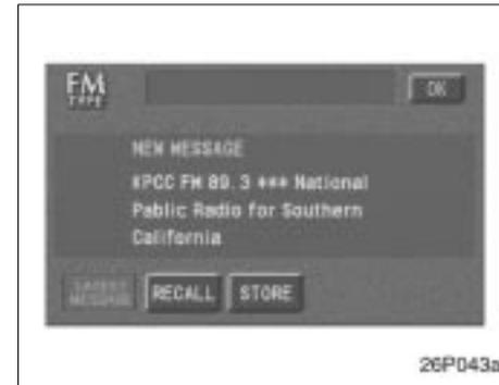
If a new message is received with the first text message on the display, "MSG" appears on the corner of the screen again. When you touch "LATEST MESSAGE", the new message appears.
