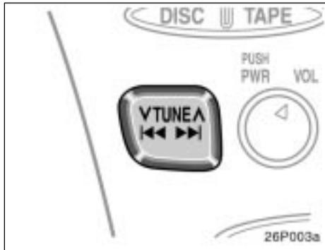
Push the “**VTUNE**” button on either side to step up the station band or to step down.
