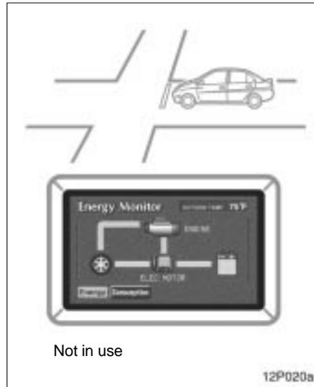
**When stopping,** the gasoline engine automatically shuts off.
