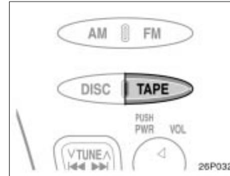
If a cassette is already in the slot, push the "DISC/TAPE" button on the "TAPE" side.
