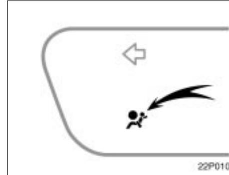
This indicator comes on when the ignition key is turned to the "ACC" or "ON" position. It goes off after about 6 seconds. This means the SRS front airbags are operating properly.
