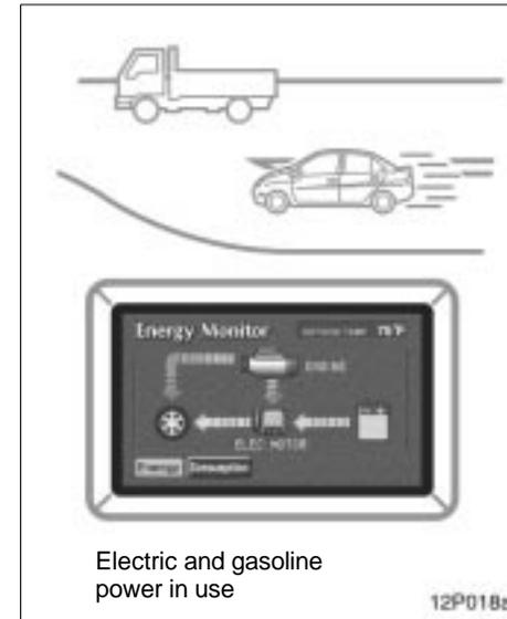
**When driving at full throttle,** electric power is further applied from the hybrid vehicle battery. Vehicle performance improves.
