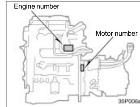
**The engine and motor number plates are installed on the engine and trans-axle case as shown.**
