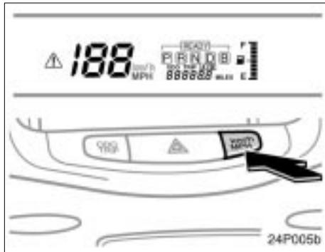
You can switch the display between km/h and MPH by pressing the button.
