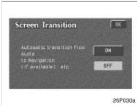
The function returning to the previous screen from the audio screen is selectable. Select "ON" or "OFF" and then touch "OK".
