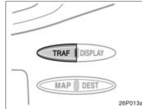
**TRAF (Traffic) function:** A station that regularly broadcasts traffic information is automatically located and broadcasts when the program starts.
