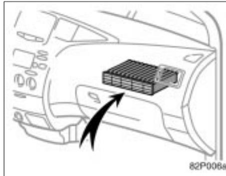
The air conditioning filter may clog after long use. The filter may need to be replaced if the air flow of the air conditioning and heater experiences extreme reductions in operating efficiency, or if the windows become to fog up easily.
