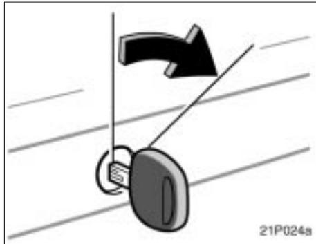
To open the trunk lid from the outside, insert the key and turn it clockwise.
