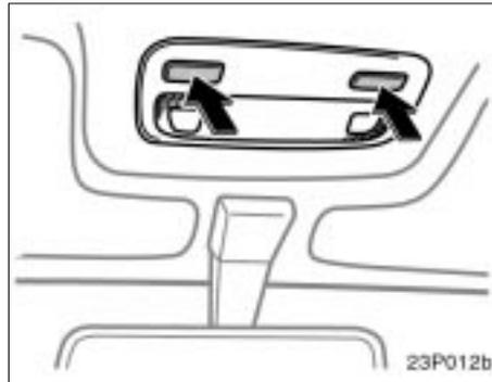
To turn on the personal light, push the switch. To turn it off, push the switch again.
