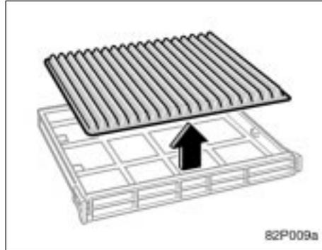
3. Remove the filter from the filter case and replace it with a new one.
