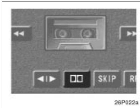
**Dolby® Noise Reduction\* feature:** If you are listening to a tape that was recorded with Dolby® B Noise Reduction, touch the switch marked with the double-D symbol. The “**DD**” switch will be highlighted in green. Touch the switch again to turn off Dolby® B NR.
