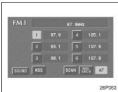
**Preset tuning:** Touch the switch (1–6) for the station you want. The switch is highlighted in green. The station frequency appears on the display.
