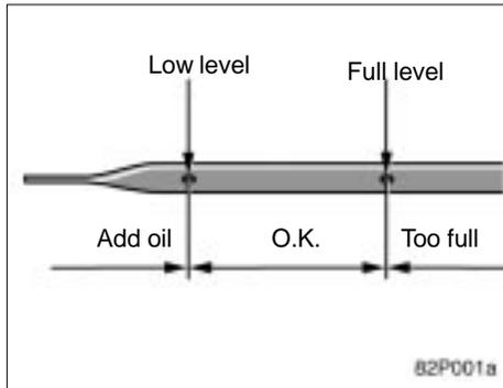
With the hybrid system at operating temperature and turned off, check the oil level on the dipstick.
